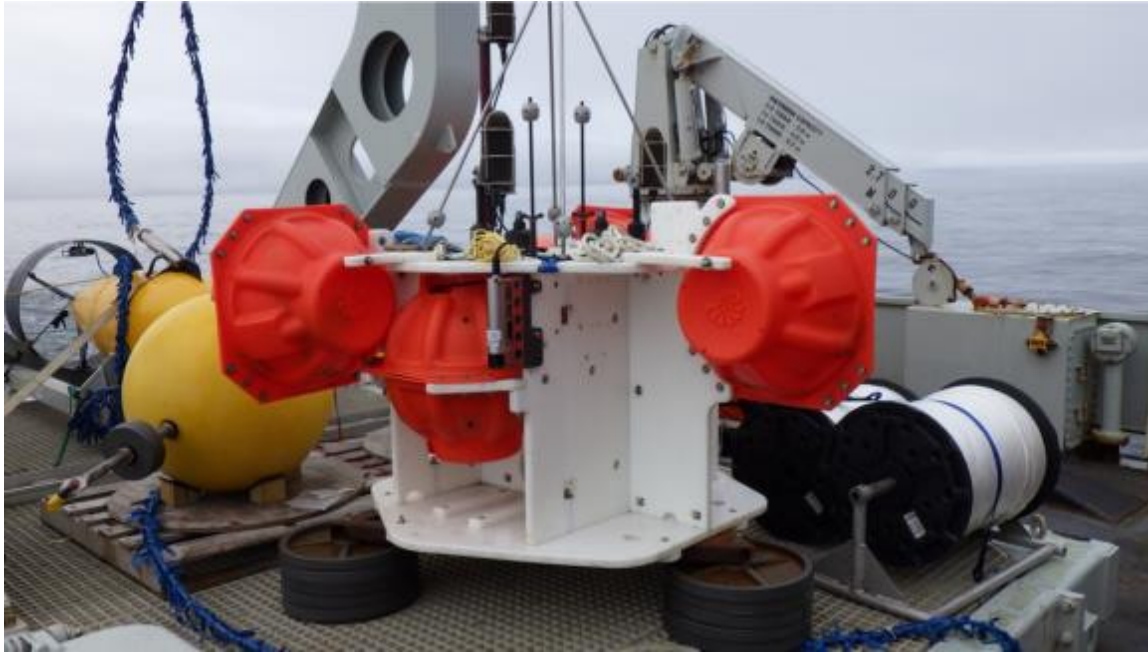
Figure 3. The ALTO-lander configuration (AMAR; JASCO) used to measure underwater sound at station AAR1.
