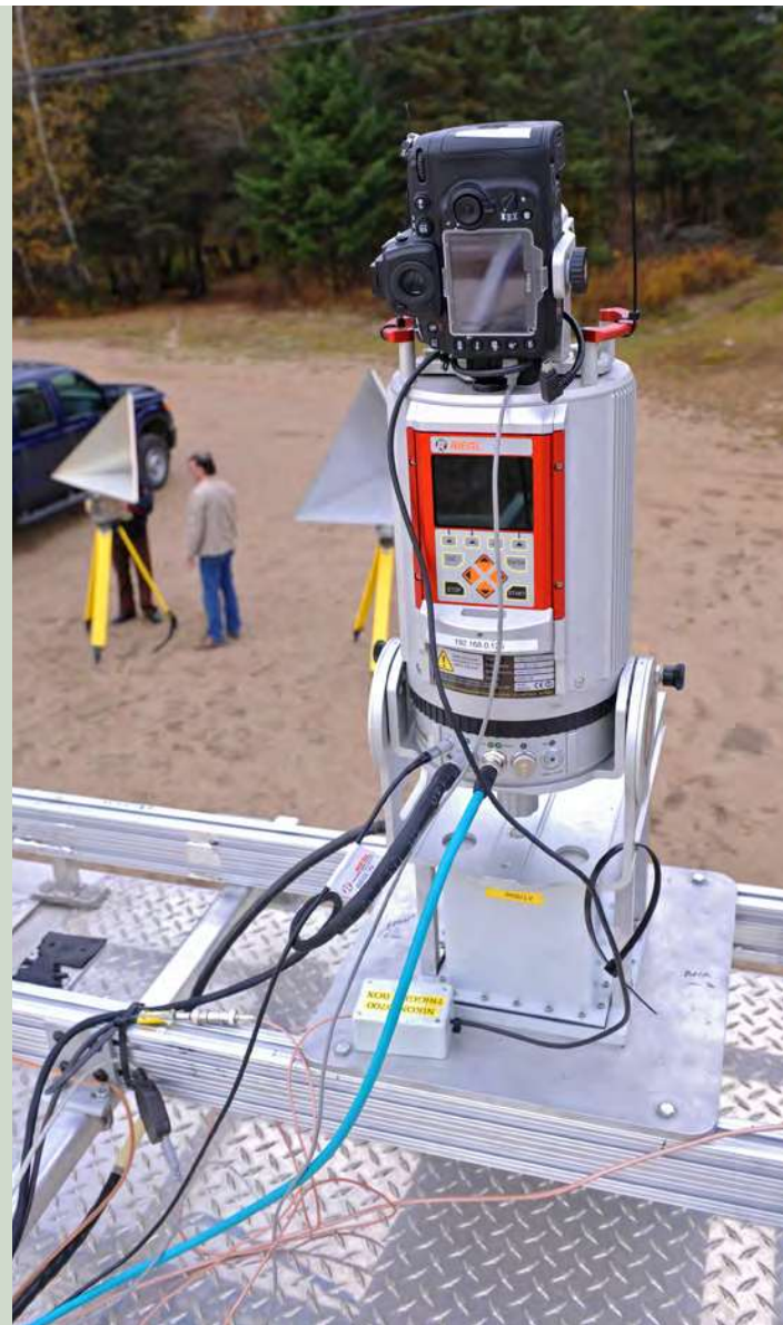
LiDAR system mounted on vehicle for testing at DRDC Valcartier.
