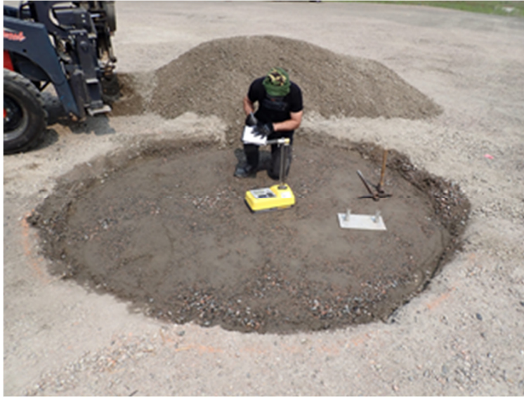
Figure 2: Measurement of the soil condition during a test site preparation using the nuclear method.
