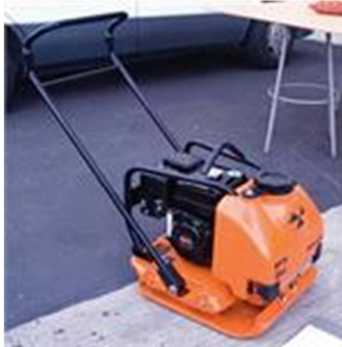
Figure 19: Small vibrating plate compactor Make: Mikasa, Model MVC88VTHW, producing 15 kN of centrifugal force.
