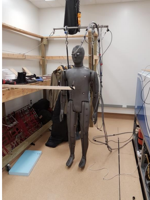
Figure 1: Thermal manikin, NEMO, in NRC TML.
