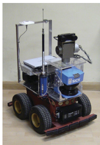
Fig. 8. The ASys robot control testbed includes construction of self-aware robot controllers [36] for mobile robot applications. The figure shows the Higgs robot, the main platform for this research [35].
