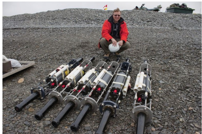
Figure 3. The array extenders and telemetry repeaters.
