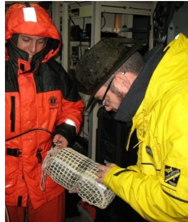
Figure 3. The Multi-Mode Pipe Projector used to emit the 189 dB/1 \mu Pa tone for the homing system.
