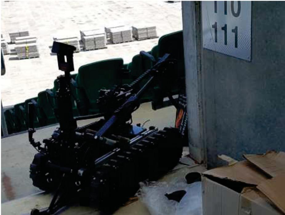
**Figure 2: RPS EDU robot retrieving the suspicious package**
