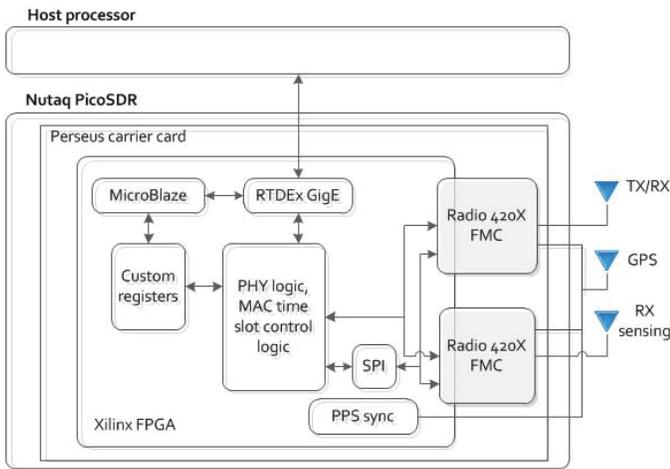
Fig. 4: SDR testbed node hardware architecture.
