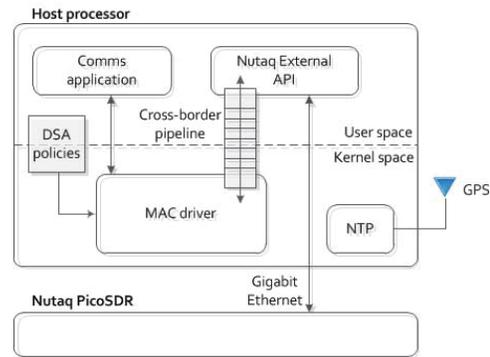
Fig. 3: SDR testbed node software architecture.
