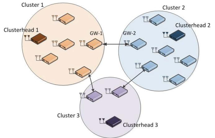
Fig. 1: Cluster-based mobile ad hoc network with gateways.
