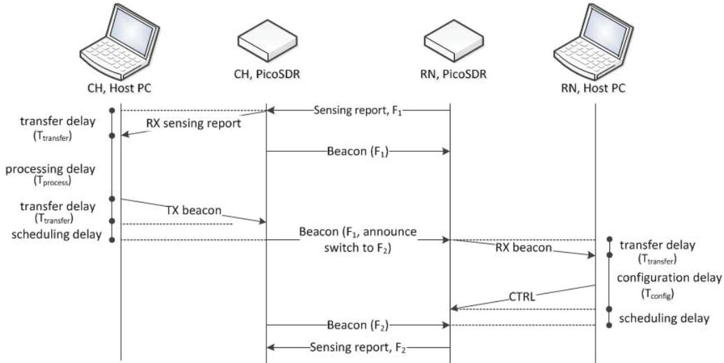
Fig. 5: Hardware and software delays in frequency switching. The scheduling delay illustrates the delay before the beacons are sent and received according to the regular TDMA schedule.
