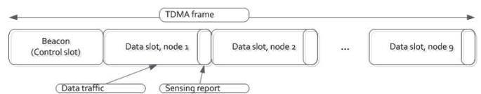
Fig. 2: TDMA frame serving a cluster of 9 nodes.
