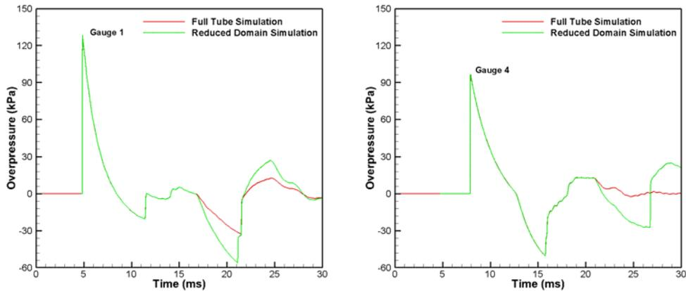
Figure 8. Comparison of reconstructed numerical waveform (reduced domain) relative to the original source (full tube simulation) (left) Gauge 1 (right) Gauge 4
