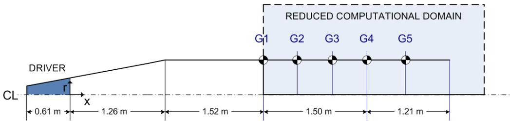
Figure 7. Schematic of reduced computational domain
