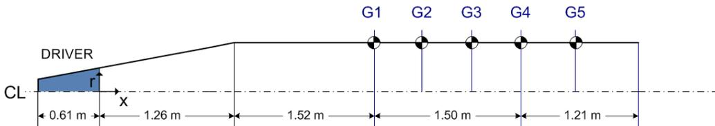
**Figure 2.** Schematic of DRDC Suffield Advanced Blast Simulator (ABS 30)
