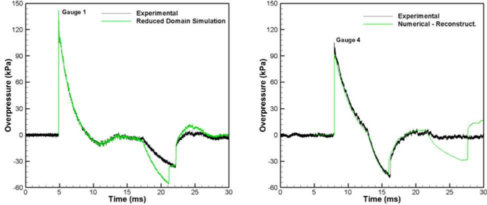
**Figure 9.** Comparison of reconstructed experimental waveform (reduced domain) relative to the original experimental measurements (left) Gauge 1 (right) Gauge 4
