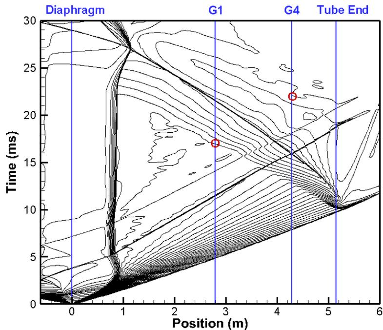
**Figure 4.** Wave diagram based on results of full tube simulation. Lines represent constant density. Circled points are referenced in Sections 4.1 and 4.3.
