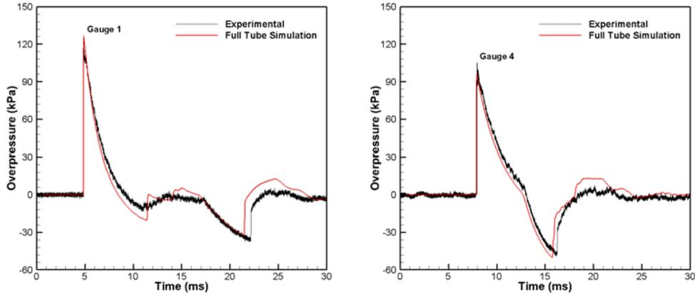
**Figure 3.** Comparison between experimental measurements and numerical predictions for simulation of full blast tube (left) Gauge 1 (right) Gauge 4
