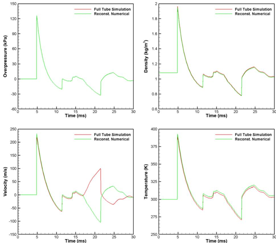
**Figure 6.** Comparison between the Gauge 1 reconstructed wave and original source (full tube simulation) at the Gauge 1 location.
