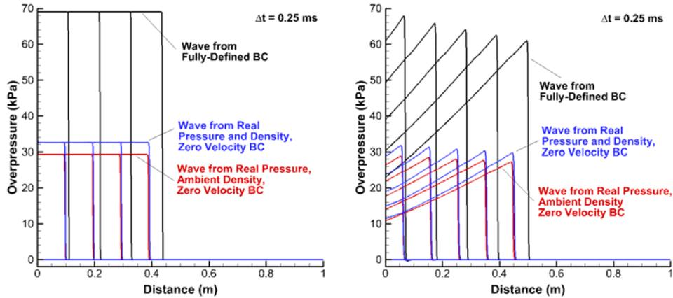
**Figure 1.** Effect of inflow boundary definition on shock propagation for (left) 69 kPa normal shock and (right) 69 kPa blast wave
