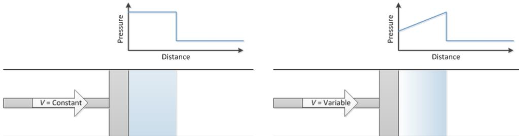
**Figure 5.** Effect of piston velocity on shock waveform produced: (left) constant piston velocity and (right) instant piston motion followed by a reduction in velocity
