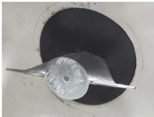
**Figure 4.** Double ended Pitot probe with static port mounted on sidewall of ABS.
