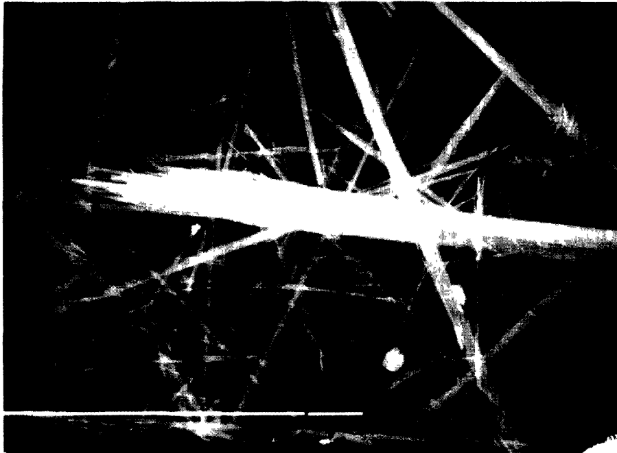
Figure 2. Typical Amosite Asbestos Fibres. (1200X)
