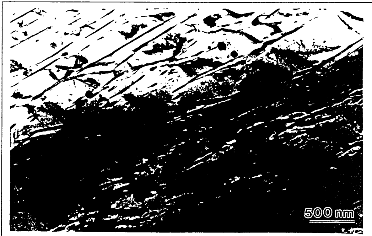
Figure 13: TEM image of a typical ( \alpha + \kappa_{III} ) eutectoid region in the reheat zone. The elongated particles are Ni-rich and have a B2 crystal structure.
