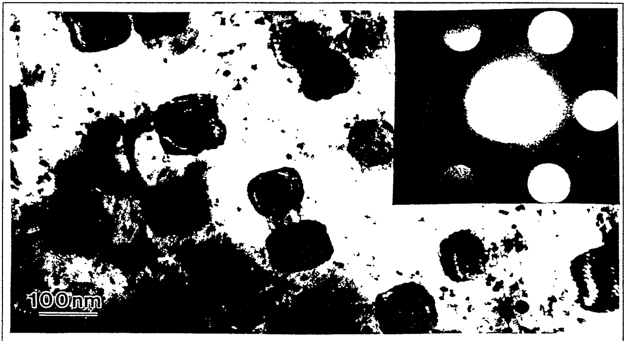
Figure 11: TEM image showing cuboidal, Fe-rich precipitates within the 9R \alpha phase. Microdiffraction patterns (inset, [111] zone axis) indicate the precipitates possess B2 crystal structure.
