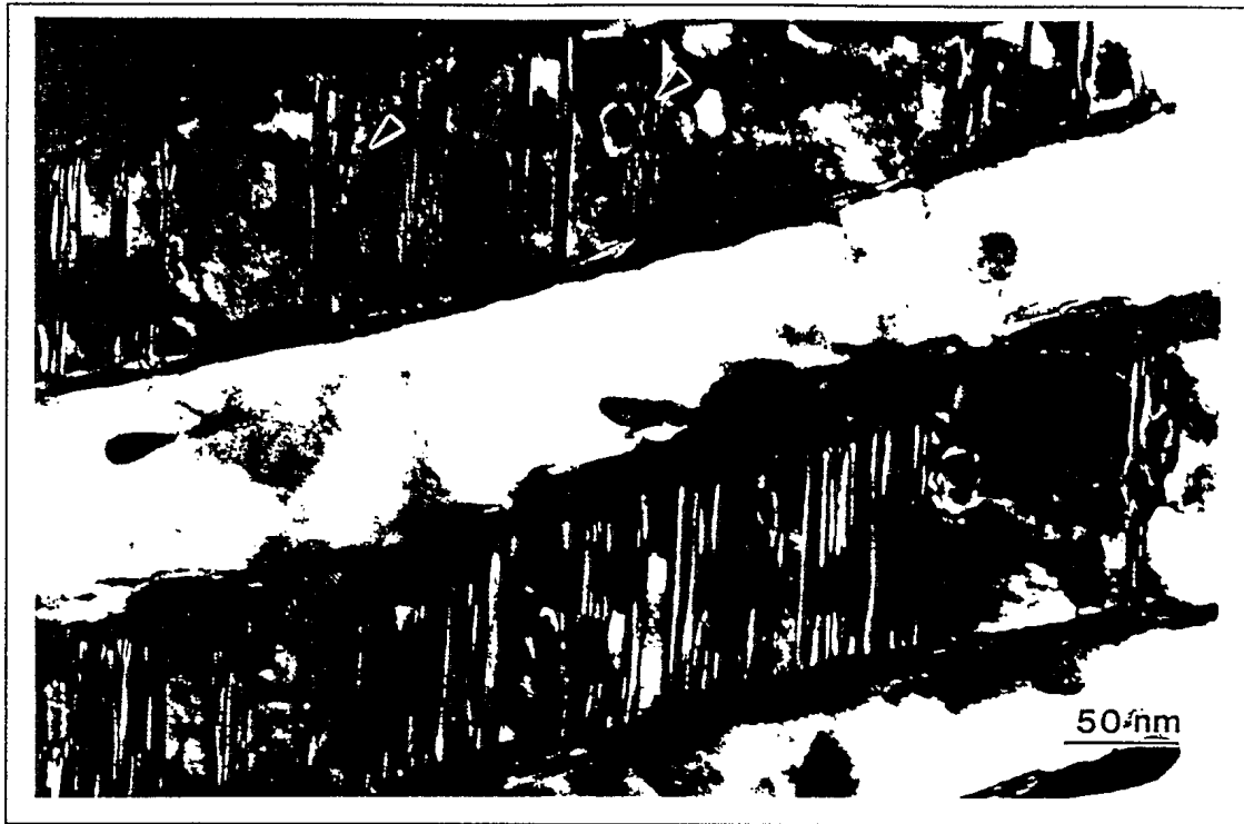
Figure 5: TEM image of a fcc \alpha rod in the as-deposited region showing clusters of stacking faults. Moire rings, arising from double diffraction, are frequently observed.
