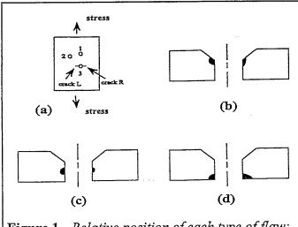
Figure 1 - Relative position of each type of flaw: ((b)-countersink, (c)-mid-bore, (d)-faying surface).
