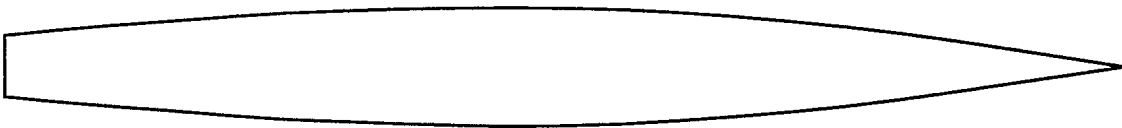
Figure 4: Waterplanes of Series 60 Ships and FFG 7
