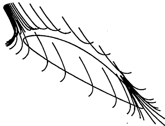
Figure 7: Cross-sections for Compound Radius Fillet Surfaces
