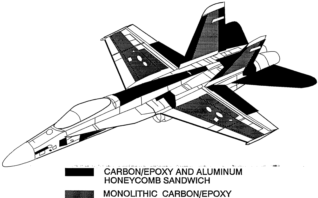
Figure 1 - Use of Composites in the CF-18
