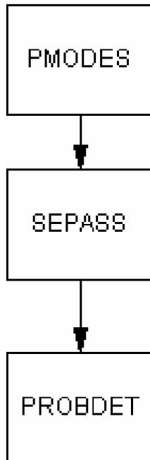
**Figure 4.** DMOS processing flow for passive sonar
