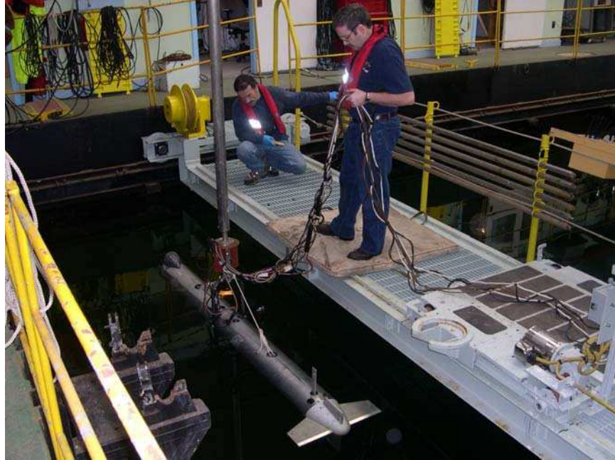
Figure 4 Tow-body on 300 lb. station for horizontal aspect characterization.
