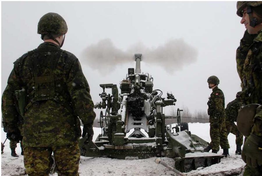
Figure 6. Emission at the muzzle end of the M777 155 mm howitzer
