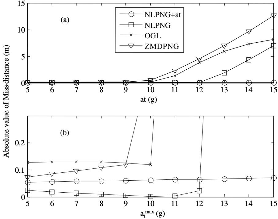
Figure 10: (a) Absolute value of miss distance for different values of  $a_t^{\max}$  (g) with  $t_f = 5$ ,  $\omega_t = 1.7$  rad/s and nominal parameters  $\bar{\omega}$  and  $\bar{\xi}$ ; (b) zoom in over [0 m, 3 m]
