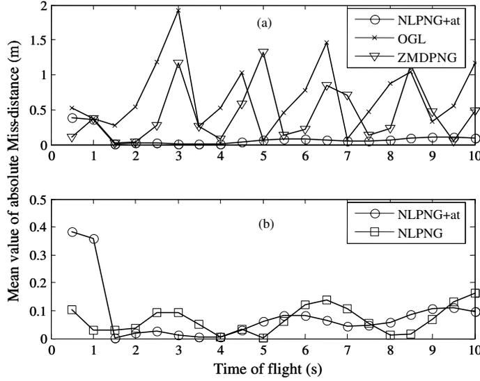
Figure 7: (a) Mean values  $E(|y(t_f)|)$  for the absolute miss distances with  $a_t^{\max} = 10g$ , and  $\omega_t = 1.7$  rad/s; (b) zoom in over  $[0 \text{ m}; 0.5 \text{ m}]$
