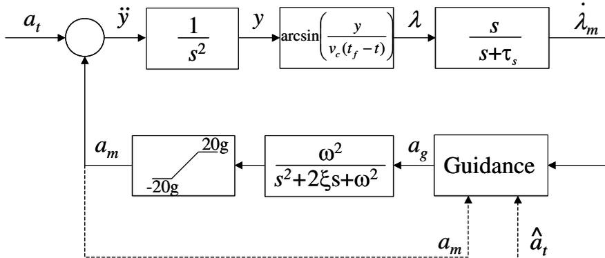
Figure 5: Block diagram of missile control system
