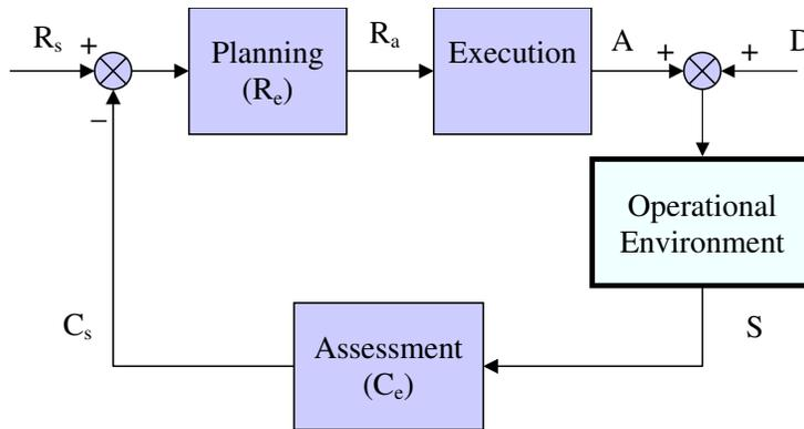
Figure 1. Block diagram of the high-level EBAO functions, variables, and feedback<sup>3</sup>
