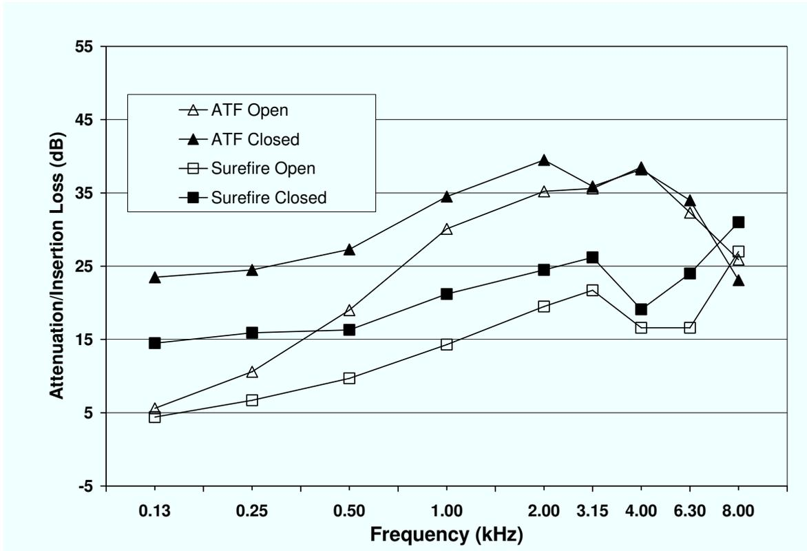
Figure 6 A comparison of results: the Surefire EP3 Sonic Defender<sup>TM</sup> versus the ATF.
