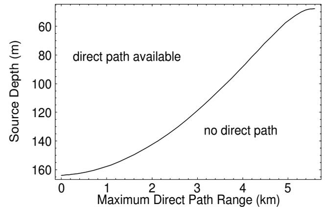
**Figure 4.** Maximum range of a direct path between a source and a receiver bottomed at 163.1 m, for the sound speed profile in Figure 1. Sources shallower than 41 m always have a direct path available.
