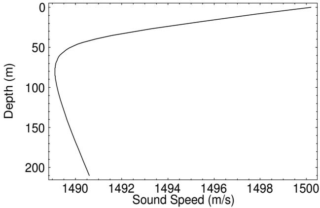
**Figure 1.** A simplified sound speed profile for the Bay of Fundy in summer. Note the upward-refracting gradient at the bottom, the location of the receivers.
