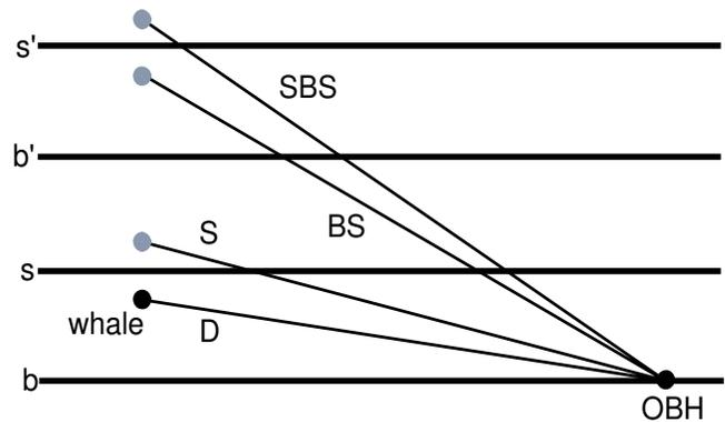
**Figure 6.** Simplified ray path analysis of arrival structure, using the image method: on the left,  $s$  and  $b$  denote sea surface and seabed, respectively;  $s'$  and  $b'$  denote images of these planes. Within the figure,  $D$  denotes a direct path with no reflections,  $S$  denotes a surface-reflected path,  $BS$  denotes a bottom-surface-reflected path, and  $SBS$  denotes a surface-bottom-surface-reflected path
