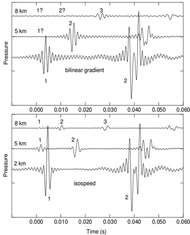
**Figure 5.** OASES model outputs of the 100-800 Hz impulse response of the shallow water channel between a shallow source and a near-bottom receiver at three ranges, including all effects of refraction, seabed interaction, and proximity of source and receiver to boundaries. Label numbers refer to arrivals in Table 2.
