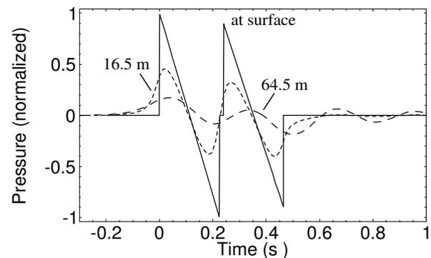
Fig. 5b: Time series of complex incident wave at three receiver depths.
