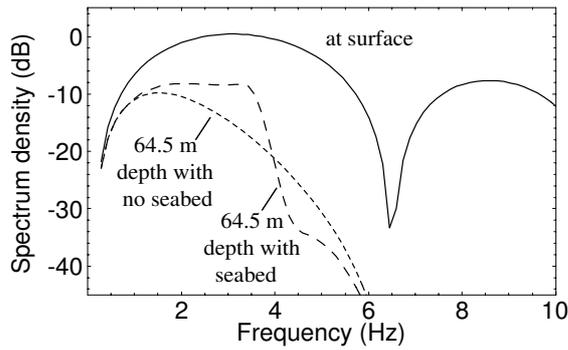
Fig. 4a: Spectrum of N-wave at surface and at 64.5 m depth, with and without a seabed at 76 m depth.
