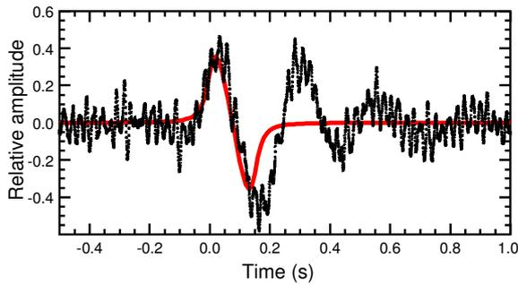
Fig. 1a: Concorde sonic boom time series recorded underwater, compared with the Sawyers-Cook model. (DC Fig. 5a)
