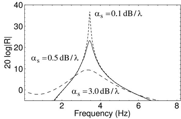
Fig. 3b: Dependence of resonance strength on shear attenuation.
