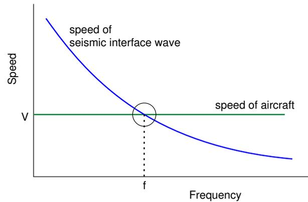
Fig. 2b: The broadband sonic boom from an aircraft travelling at speed  $V$  could excite a seismo-acoustic interface wave at the frequency where their speeds coincide.
