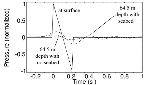
Fig. 4b: Time series of N-wave at surface and at 64.5 m depth, with and without seabed interaction.
