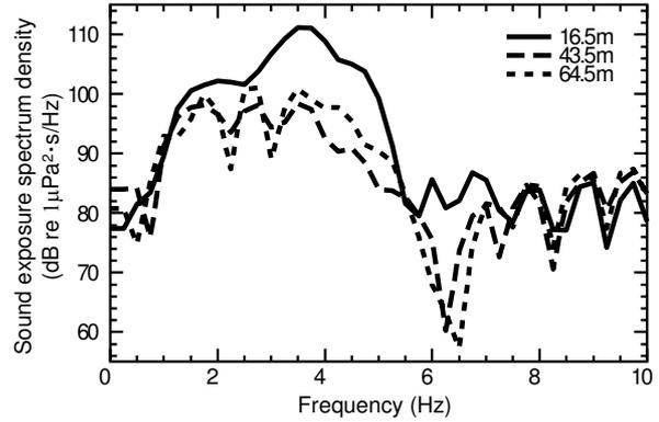
Fig. 1b: Concorde sonic boom spectrum measured at three depths. (DC Fig. 7)
