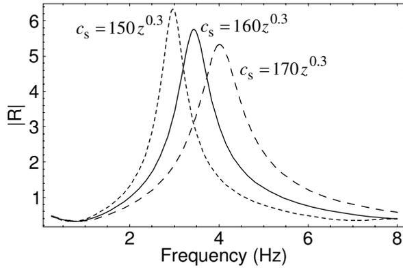
Fig. 3a: Dependence of resonance frequency on shear speed profile for a Mach 2 source.
