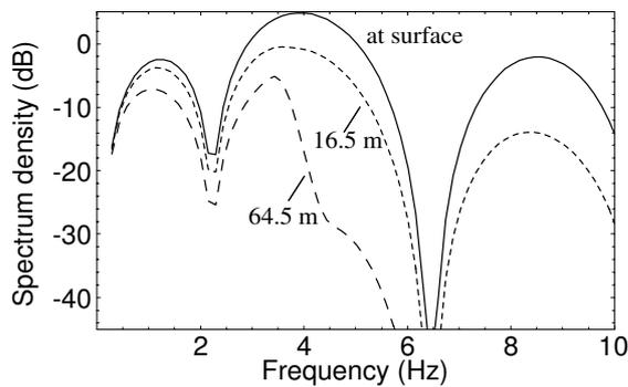
Fig. 5a: Spectrum of complex incident wave at three receiver depths.
