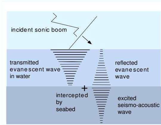
Fig. 2a: Schematic of the proposed enhancement mechanism.
