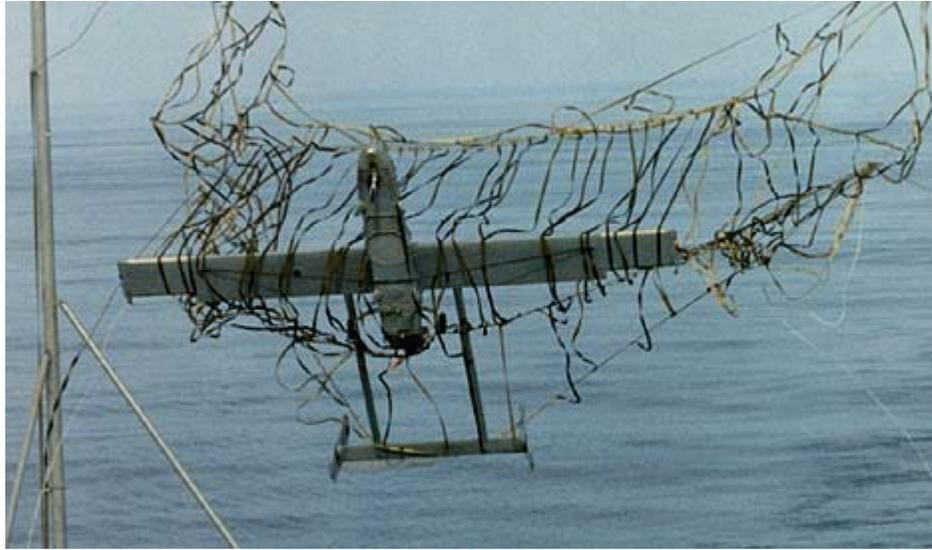
*Figure 4: The Pioneer UAV being retrieved with a net [10].*
