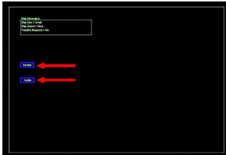
Figure 3. Screen capture of the modified Status display. The red arrows indicate the “neutral” and “hostile” buttons.
