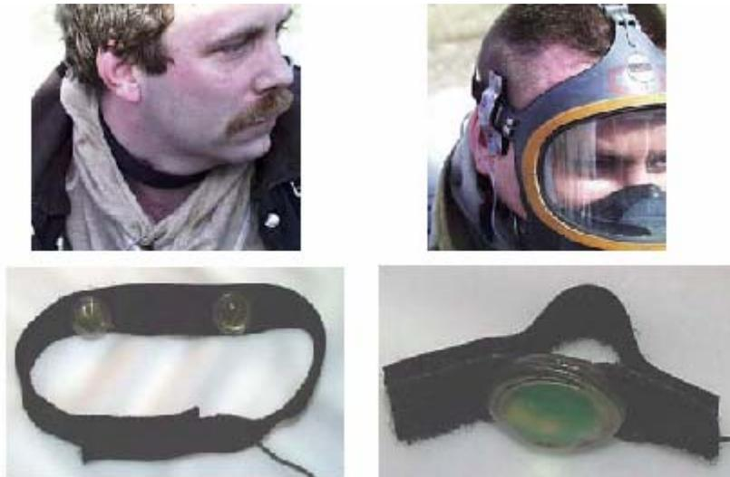
**Figure 5. Physiological Microphone Neckstrap (top left), Goggle Mount (top right), Neckstrap Detail (bottom left), and Goggle Mount Detail (bottom left).**
