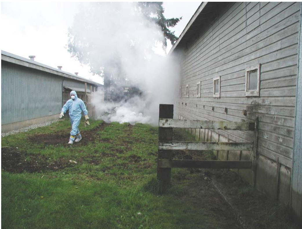
Figure 3. Demonstration of airflow characteristics using a smoke model
