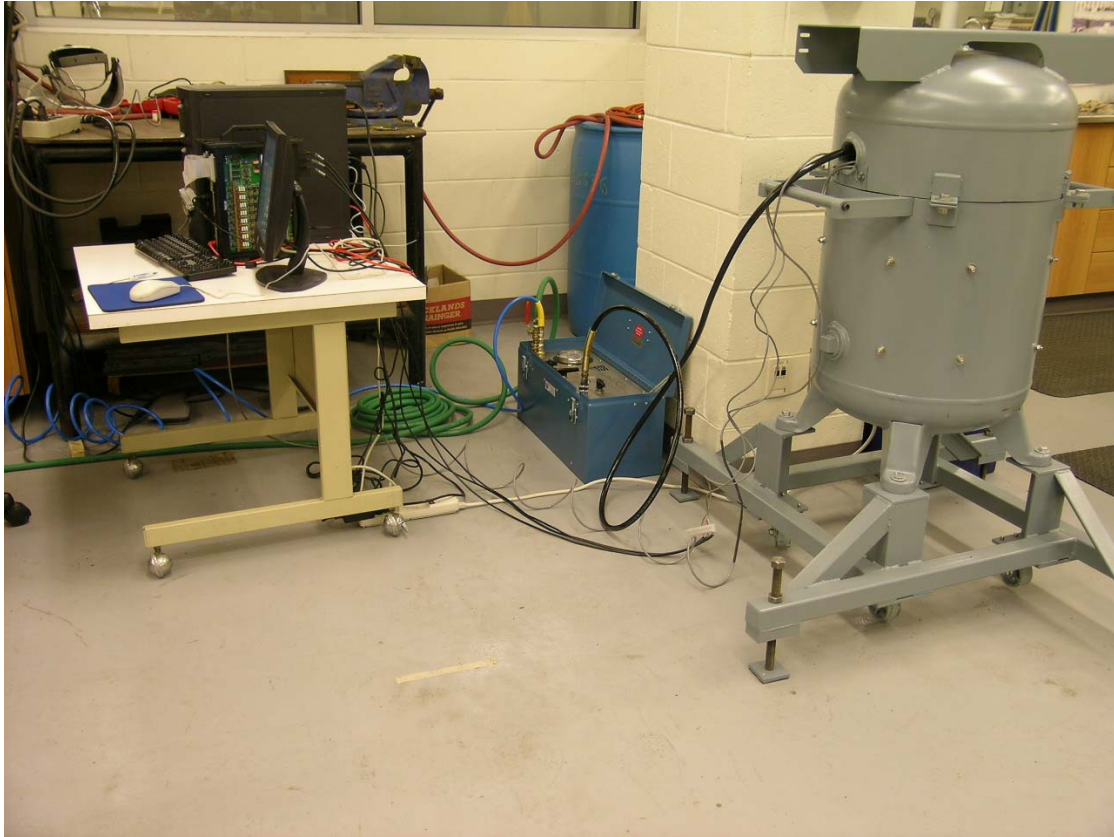
Figure 3.2. Photograph showing the functional relationship between the containment chamber, the pump, and the data acquisition electronics for a fully configured test.
