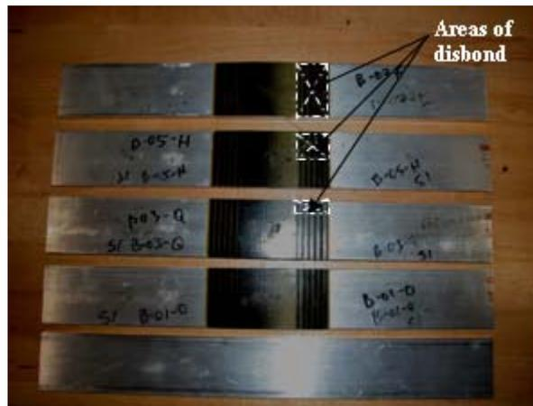
Figure 8: The five Al 6061-T651 tested specimens.
