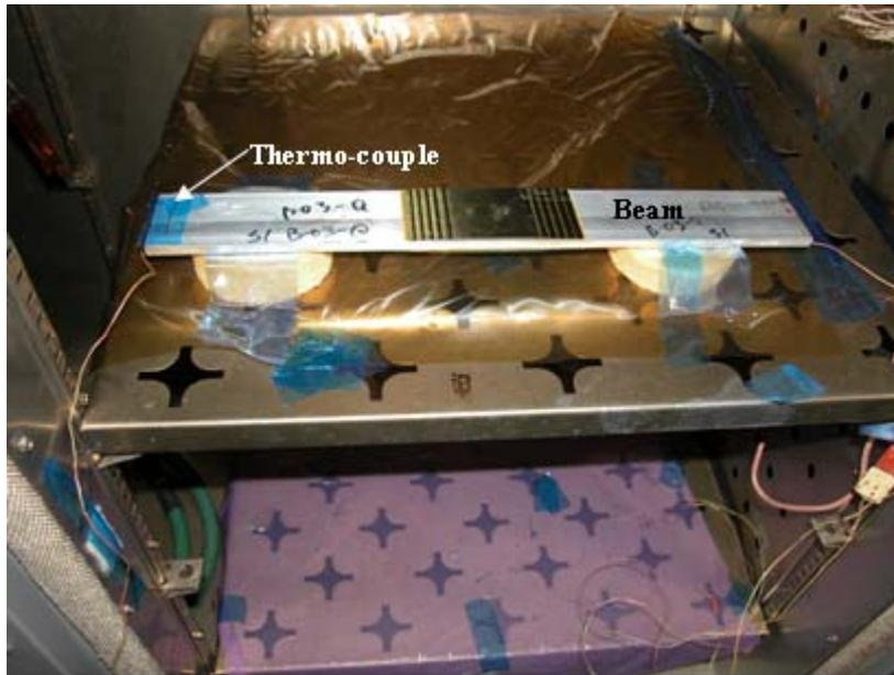
*Figure 20: Placement of the beam in the thermal environment (oven). B03 beam is shown with the thermo-couple attached.*
