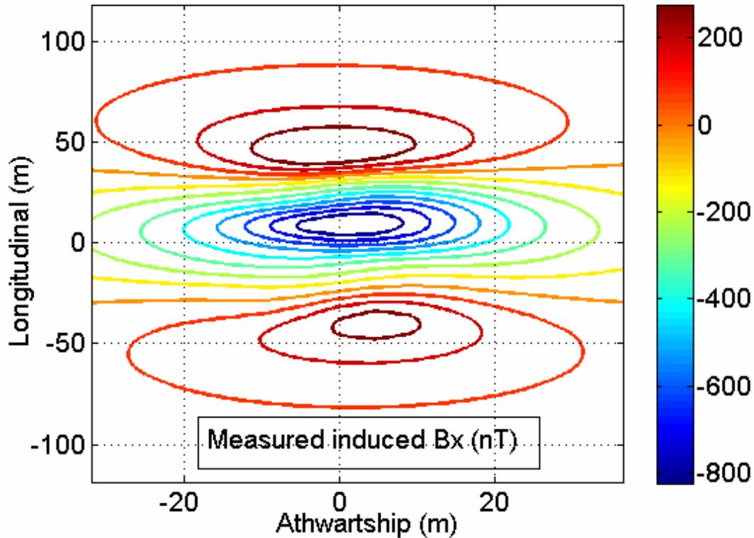
**Figure 3 (b).** Induced  $I_x^X$  signature from measurements (equation 7).
