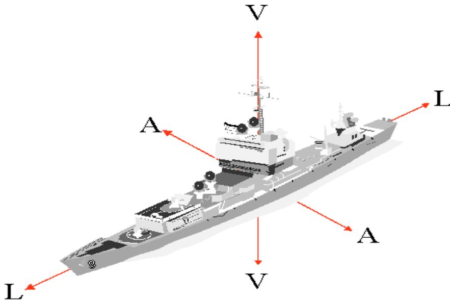
*Figure 1. Coordinate system of the ship's magnetization.*
