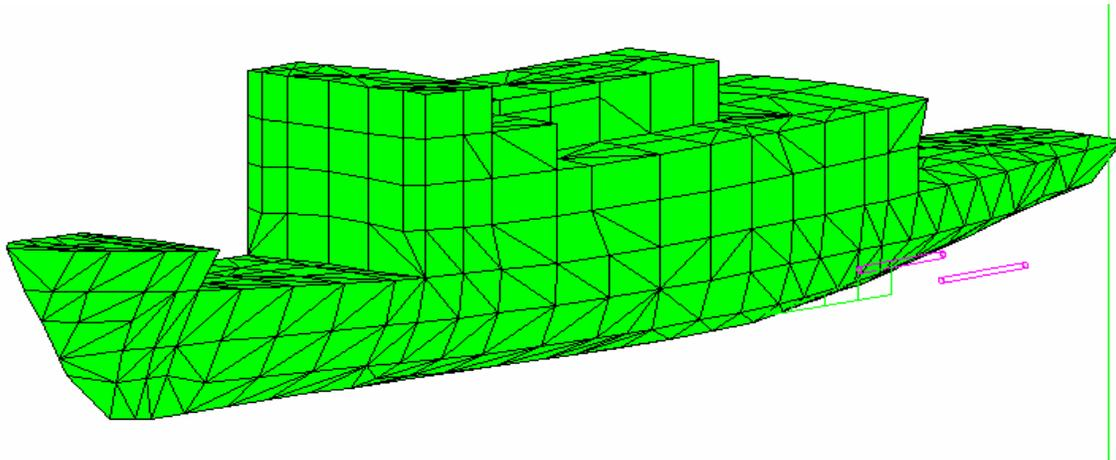
**Figure 2.** FE model of the CFAV Quest.
