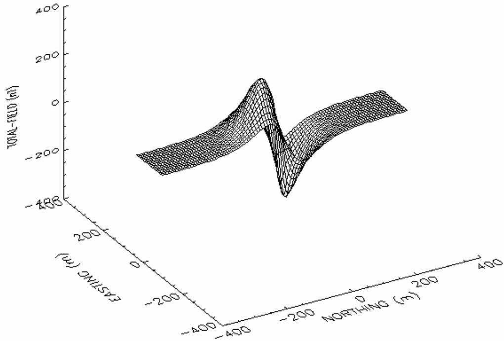
Figure 4c. Total-field anomaly due to vertical permanent magnetization only, ship heading =  $180^\circ$  (True), aircraft altitude=80 m.
