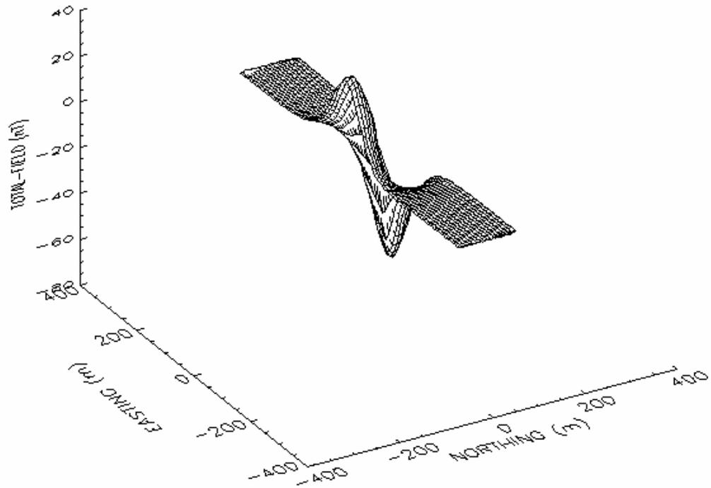
Figure 3b. Total-field anomaly due to induced magnetization only, ship heading = 90° (True), aircraft altitude=80 m.
