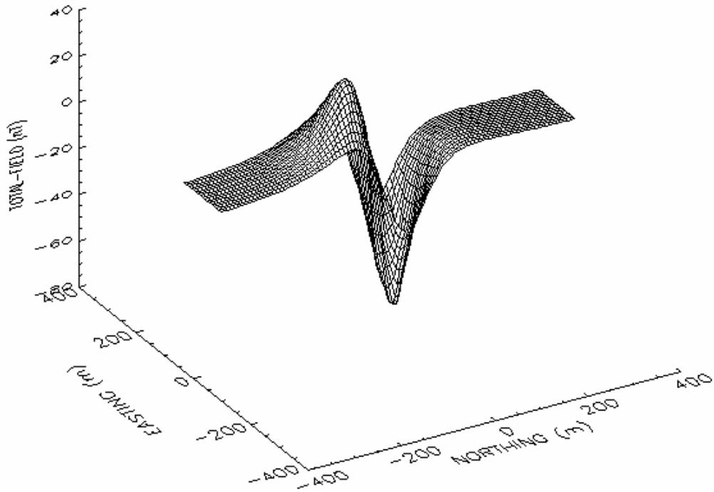
Figure 3c. Total-field anomaly due to induced magnetization only, ship heading = 180° (True), aircraft altitude=80 m.
