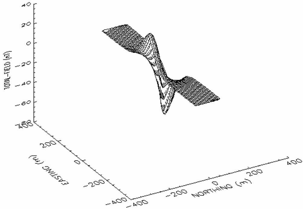
Figure 3d. Total-field anomaly due to induced magnetization only, ship heading = 270° (True), aircraft altitude=80 m.
