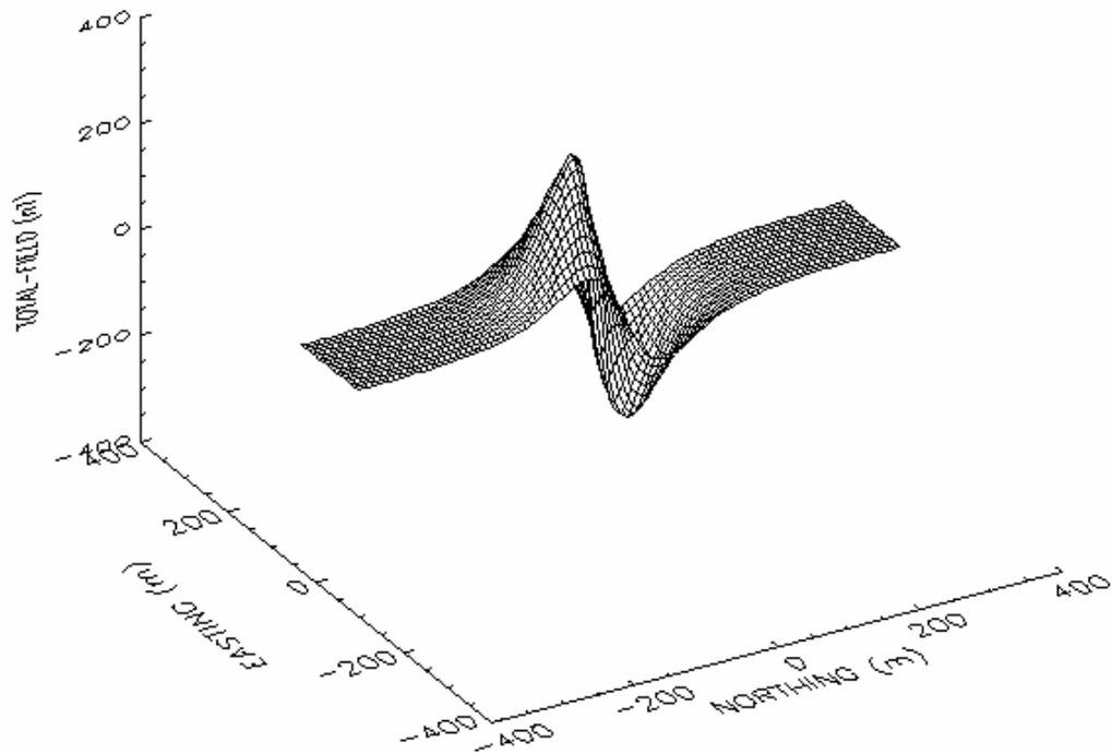
Figure 4a. Total-field anomaly due to vertical permanent magnetization only, ship heading =  $0^\circ$  (True), aircraft altitude=80 m.
