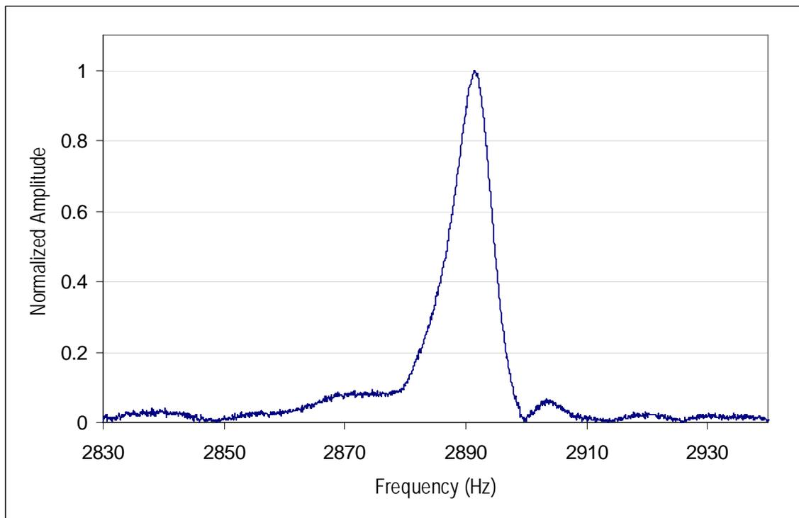
*Figure 17: A sample of the 5<sup>th</sup> natural frequency response obtained employing the experimental set up described herein.*
