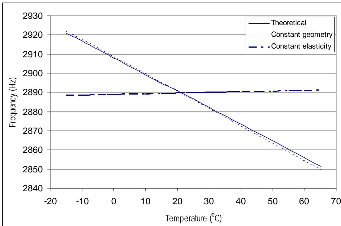
Figure 14: A comparison of the 5<sup>th</sup> natural frequencies obtained for the theoretical, constant geometry and constant elasticity models.
