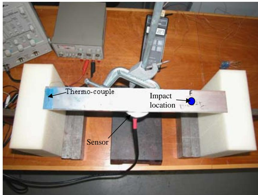
Figure 19: The final positioning of the aluminum beam on the foam supports with the sensor beneath it. The placement of the thermo-couple is also shown.
