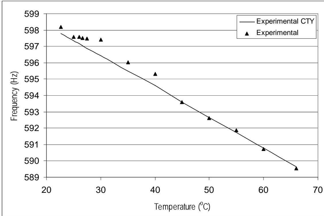
Figure 23: The variation of the 2<sup>nd</sup> natural frequency as a function of temperature.
