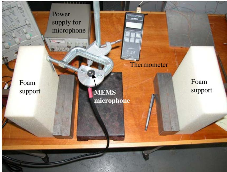
Figure 18: An overview of the experimental setup used for the temperature measurements.
