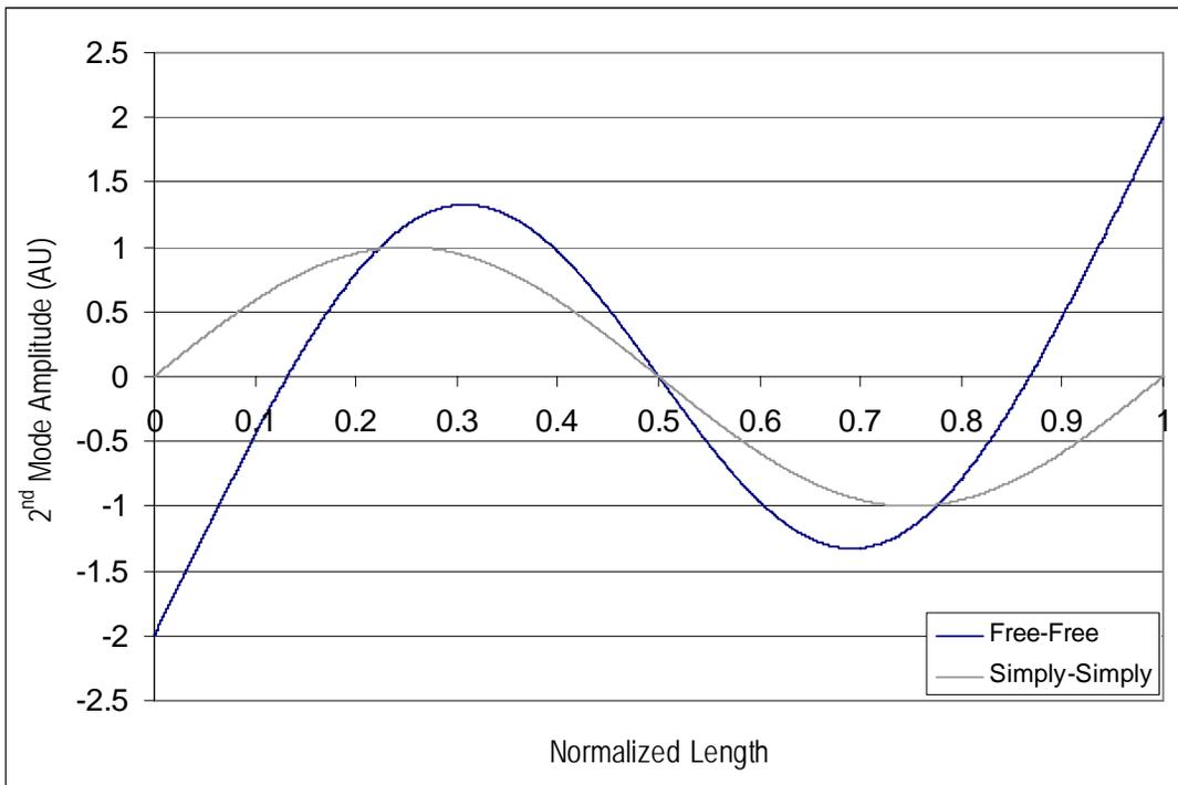
Figure 4: A comparison of the 2<sup>nd</sup> flexural mode deflection for free-free and simply-simply boundary support conditions, respectively.
