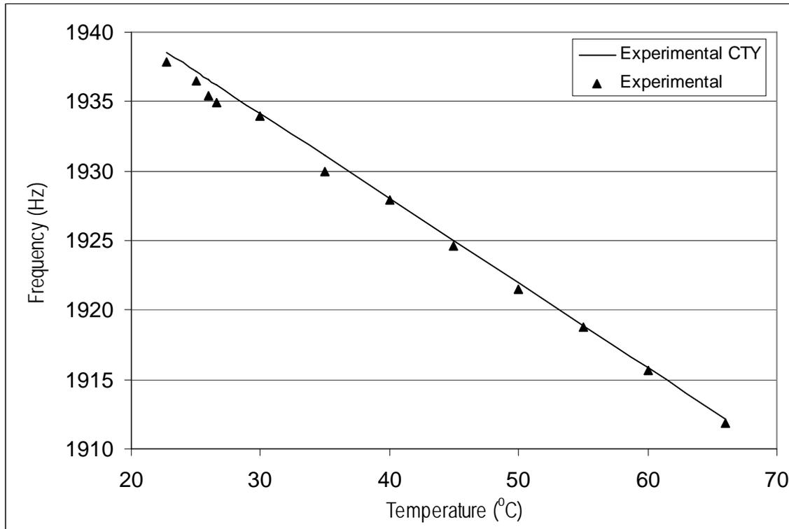
Figure 25: The variation of the 4<sup>th</sup> natural frequency as a function of temperature.
