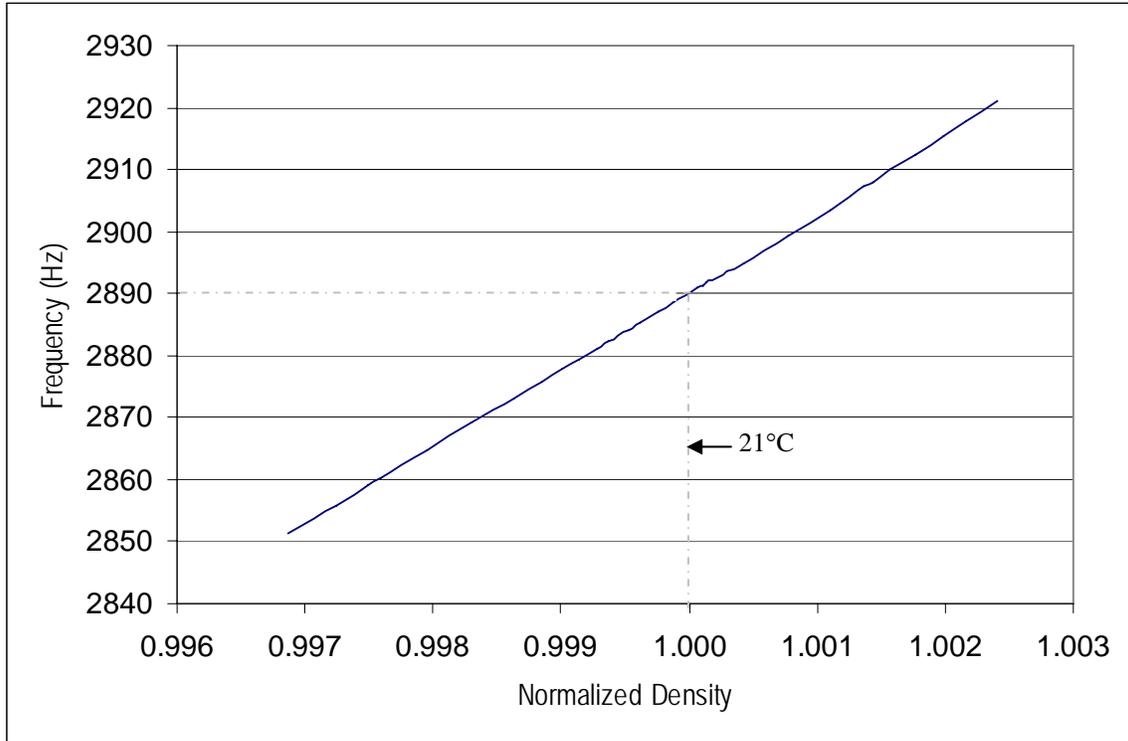
Figure 9: The effect of thermally dependent density on the natural frequency of the aluminum beam.
