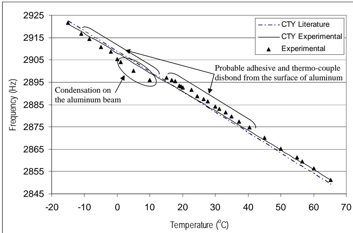
Figure 22: Changes in the 5<sup>th</sup> resonance frequency as a function of temperature. Experimental and theoretical results are compared. Highlighted areas indicate adhesive and thermo-couple disbond from the aluminum surface. Condensation effects are also indicated.
