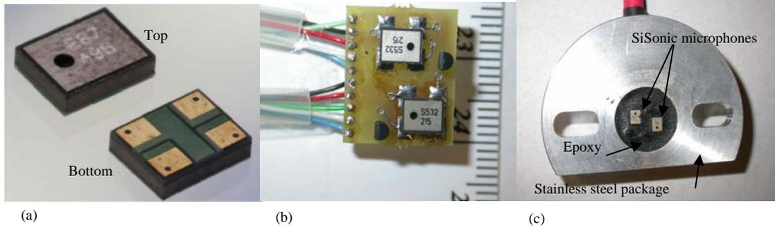
Figure 1: (a) SiSonic microphones. (b) Circuit board layout. (c) Final pressure sensor assembly showing two sensors.
