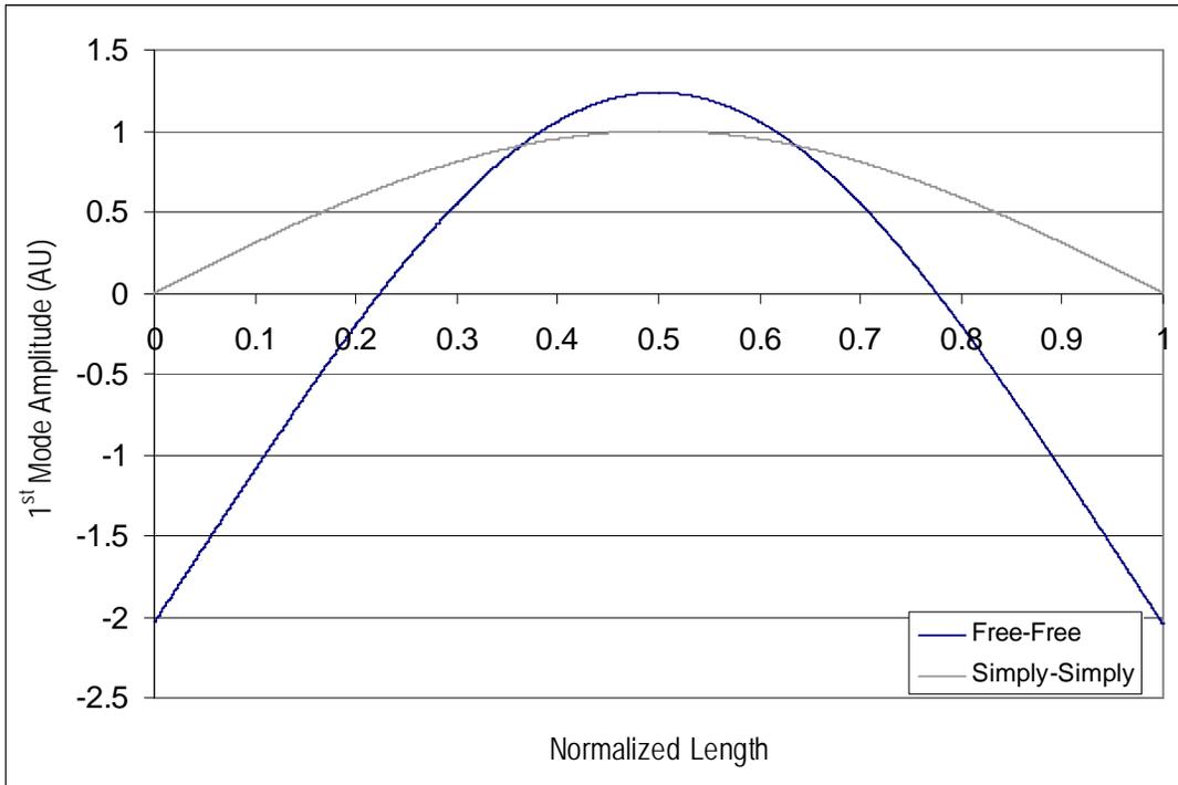
Figure 3: A comparison of the 1<sup>st</sup> flexural mode deflection for free-free and simply-simply boundary support conditions, respectively.
