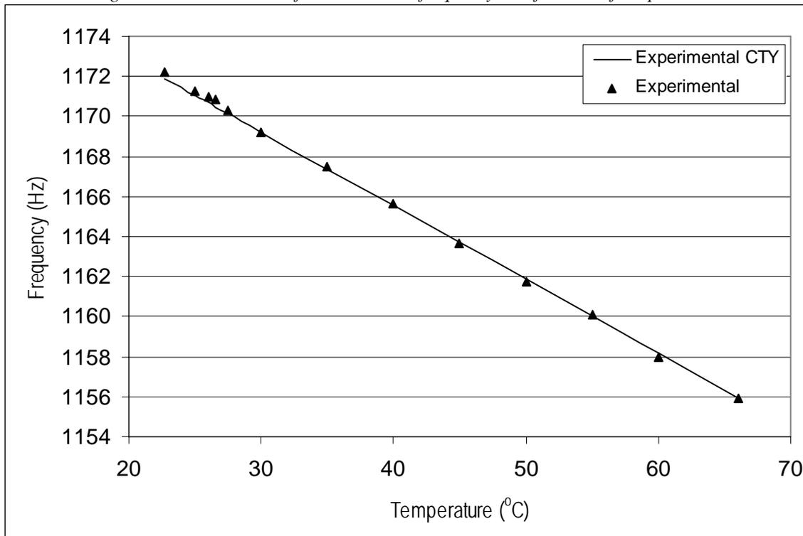
Figure 24: The variation of the 3<sup>rd</sup> natural frequency as a function of temperature.
