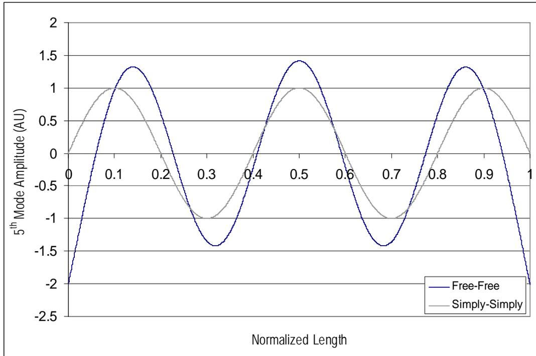
Figure 7: A comparison of the 5<sup>th</sup> flexural mode deflection for free-free and simply-simply boundary support conditions, respectively.
