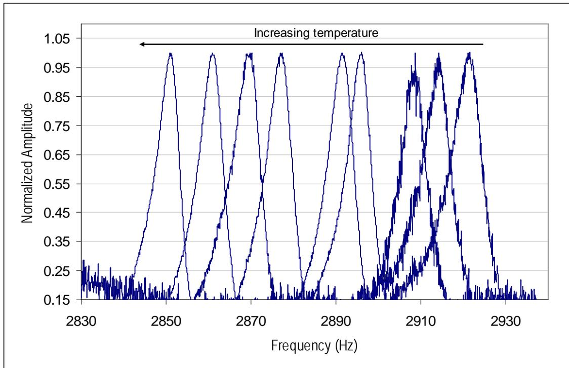
Figure 20: The shift to lower frequency of the 5<sup>th</sup> natural frequency as a function of increasing temperature.
