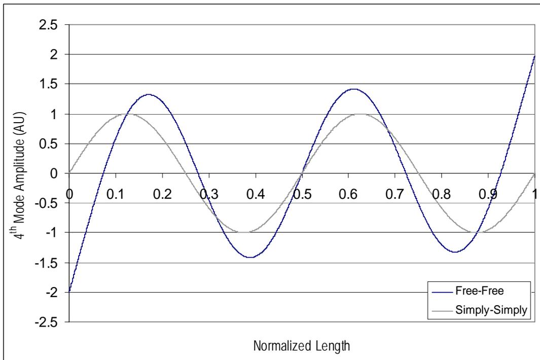
Figure 6: A comparison of the 4<sup>th</sup> flexural mode deflection for free-free and simply-simply boundary support conditions, respectively.
