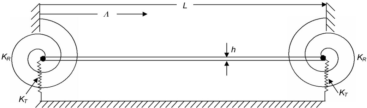
Figure 2: Artificial spring model for varying the boundary support conditions between *free-free* and *simply supported-simply supported*.
