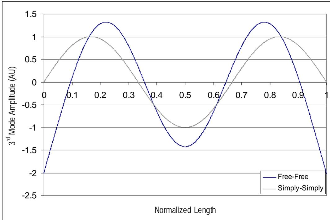
Figure 5: A comparison of the 3<sup>rd</sup> flexural mode deflection for free-free and simply-simply boundary support conditions, respectively.
