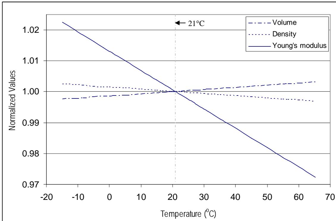
Figure 11: The changes in normalized volume, density and young's modulus as a function of temperature.
