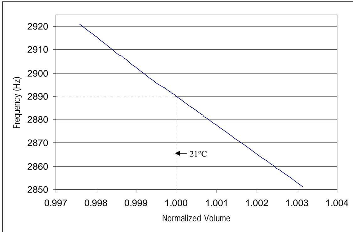
Figure 8: The variation of the natural frequency as a function of the thermally dependent volume.
