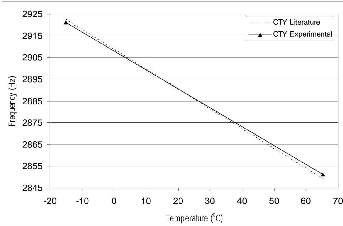
Figure 21: A comparison of the coefficients of thermal dependence for Young's modulus (CTY) found in the literature and the experimentally obtained value.
