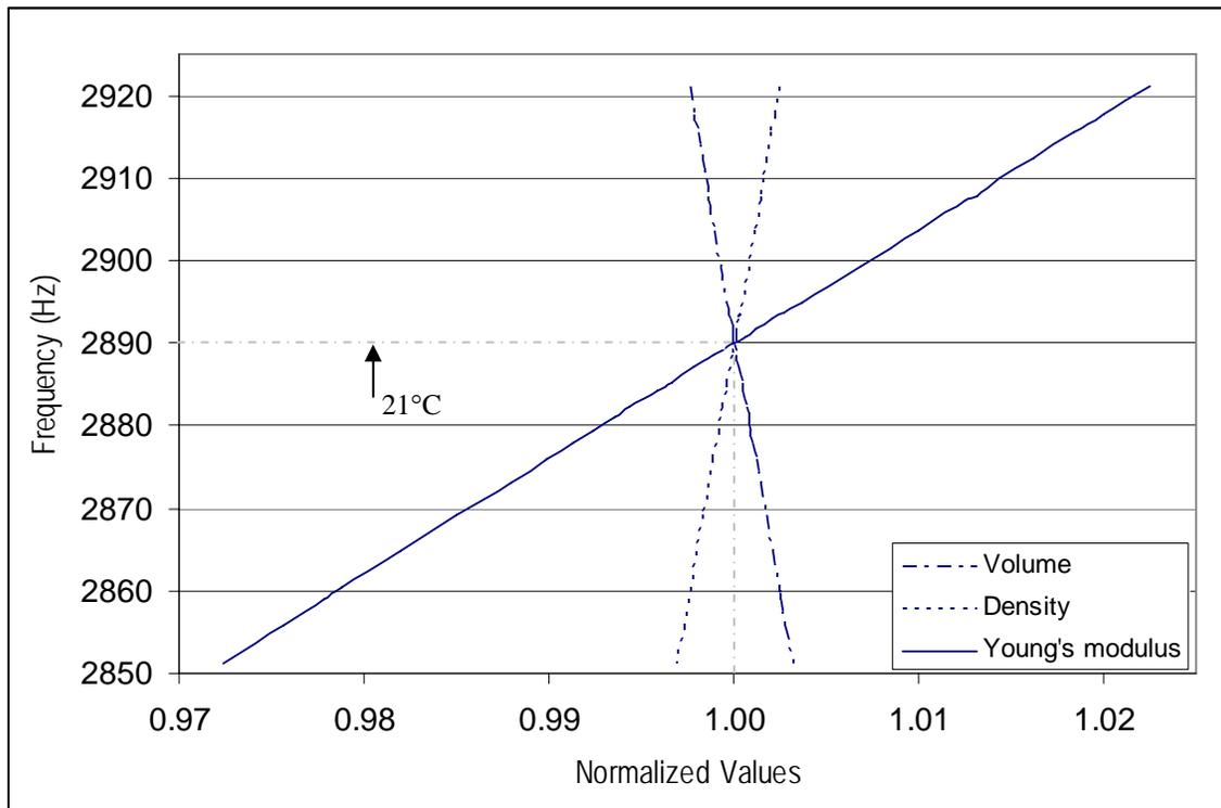
Figure 12: A comparison of the variation in frequency as a function of the normalized physical values.
