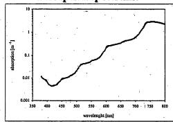
The absorption coefficient of pure water at 22°C as a function of wavelength from 380 nm to 800 nm. The solid line is the fit using a set of Gaussians whose parameters are given in Table 1 and the dots are the experimental data of (Pope and Fry 1997: 380 to 727.5 nm, Kou et al. 1993: 728 to 800 nm). Note the broad quadratic shaped minimum around 420 nm.
