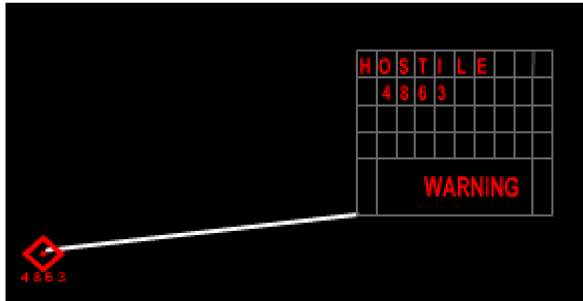
Figure 5: The tooltip that corresponds to the hostile surface contact. It remains in one location for a pre-determined length of time with a line connecting the tooltip to the active contact.
