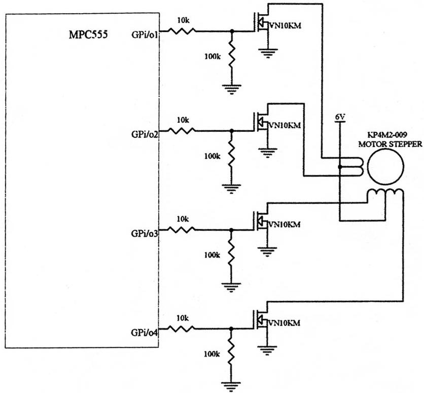
**Figure 4: Electrical scheme of the stepper motor driver.**
