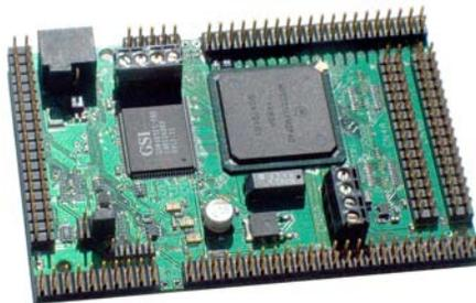
*Figure 3: SS555-DK development kit provided by Intec Automation Inc.*
