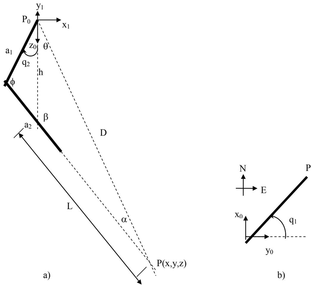
**Figure 12: Geometry of the system with corresponding variables for the DGPS waypoint tracking algorithm: a) x-z view and b) x-y view.**
