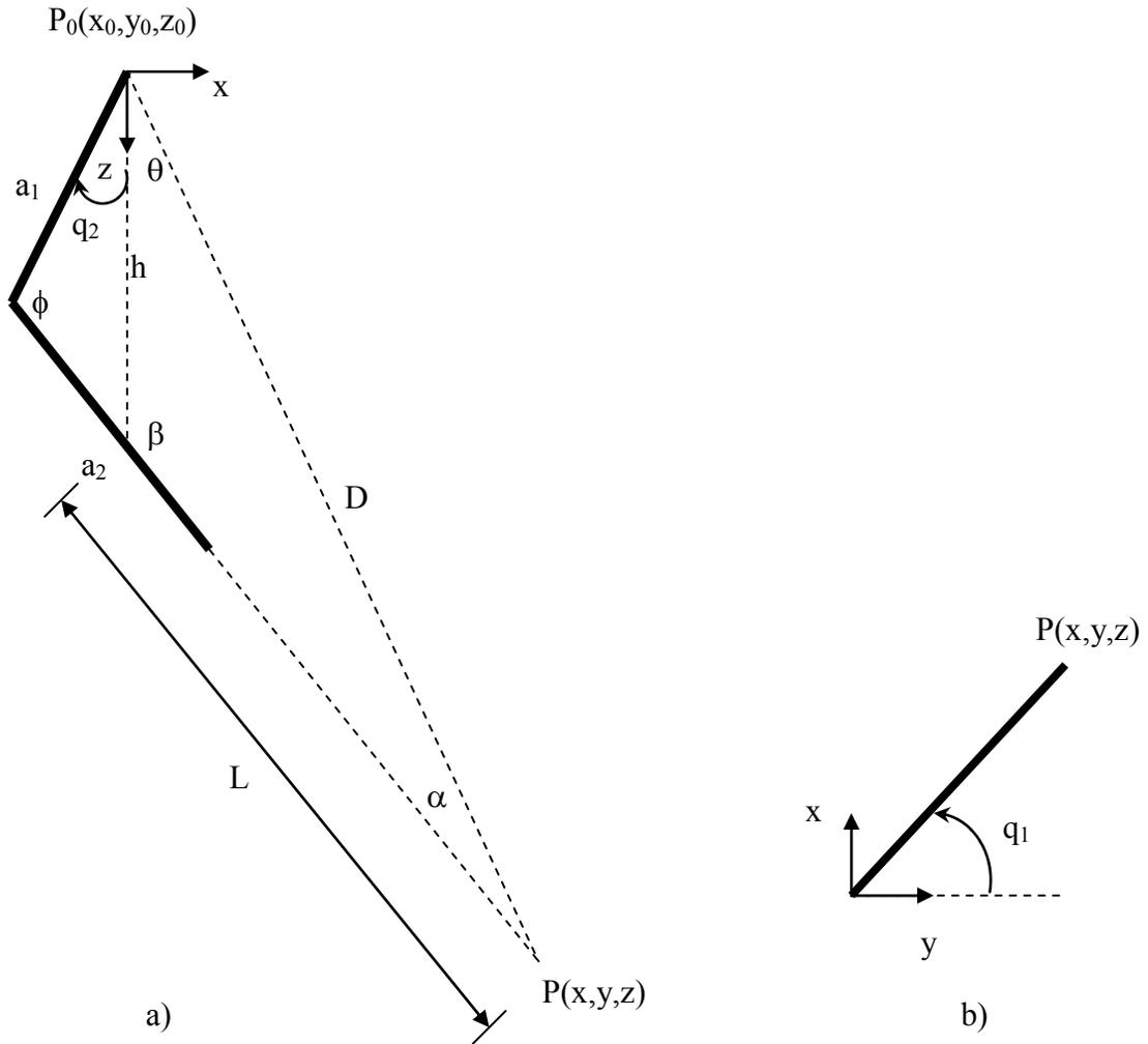
**Figure 8: Geometry of the system with corresponding variables: a) x-z view and b) x-y view.**
