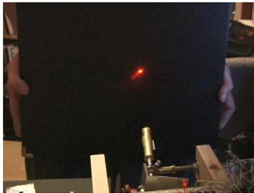
*Figure 10: A laser pointer is substituted to the camera to validate the Cartesian-space trajectory planning algorithm.*
