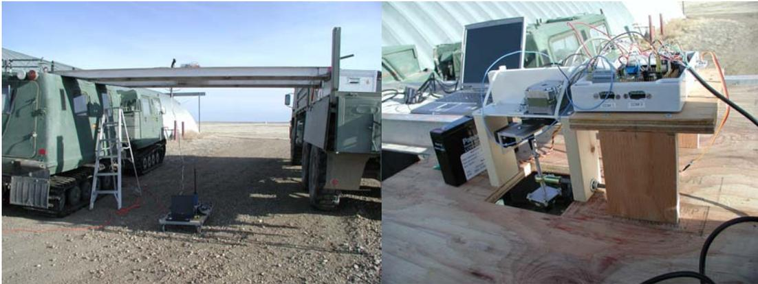
**Figure 11: GPS experiment setting. The DGPS system is moved on the ground and the camera system tracks it from a high platform. It was noticed that no satellite was seen when the system was between the two trucks so the trucks were replaced by ladders.**
