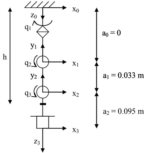
Figure 5: Robot frames representation.
