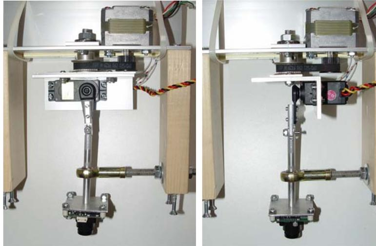
*Figure 2: Face and side view of the camera mechanism.*
