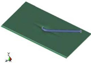
*Figure 2 Yaw and bending of a short rod by a near field blast*
