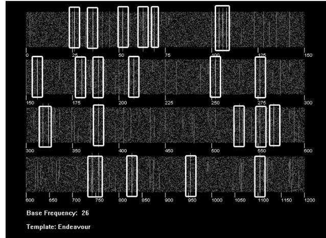
Figure 3: Sonar display with ID template overlaid
