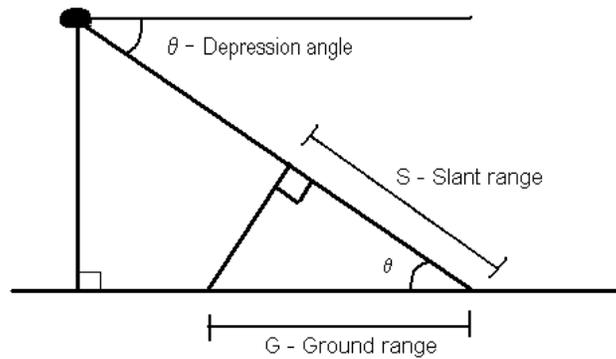
Figure 3: Representation of slant range and ground range.
