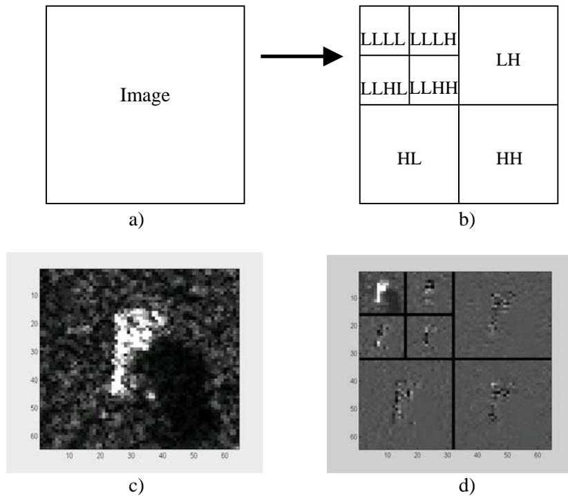
Figure 8: Two level decomposition of discrete wavelet transform. a) Block representation of an image. b) Block Wavelet representation of second resolution levels. c) Original BMP2 image. d) The BMP Wavelet representation of second resolution levels.
