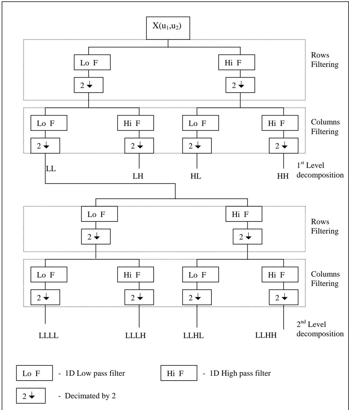
Figure 7: Pyramidical tree structure two levels of 2D wavelet decomposition steps for images.
