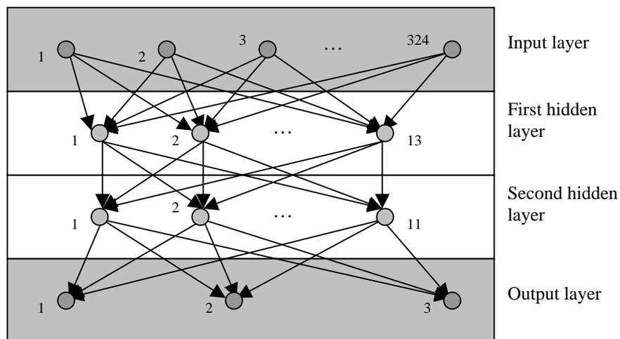
Figure 10: Four layer Multi Layer Perceptron Neural Network.
