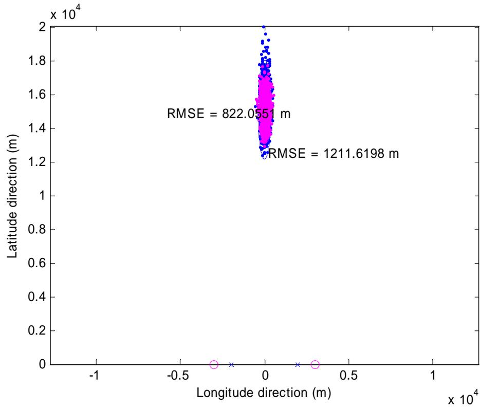
Figure 9: Comparison of emitter location estimates for two receiver pair separations. The emitter is at 15 km from the midpoint of the line joining the two receiver pairs. The “x” plot symbols mark the two receiver pairs separated by 4 km; the 1000 estimates and the 95% concentration ellipse are in blue. The “o” plot symbols indicate the two receiver pairs separated by 6 km; the corresponding 1000 estimates and the 95% concentration ellipse are in magenta.
