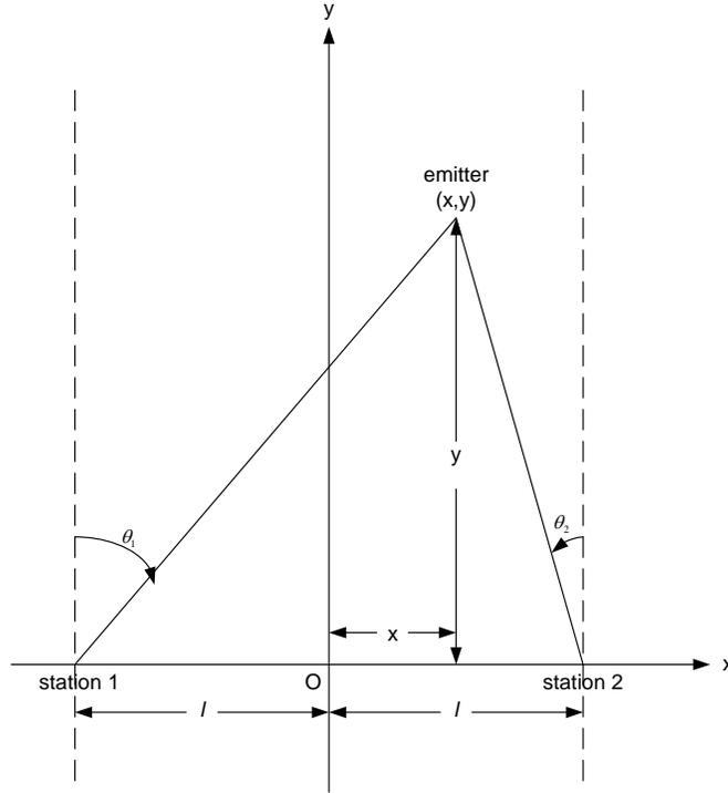
Figure 10: Two-dimensional emitter geolocation based on bearings measured by two stations.
