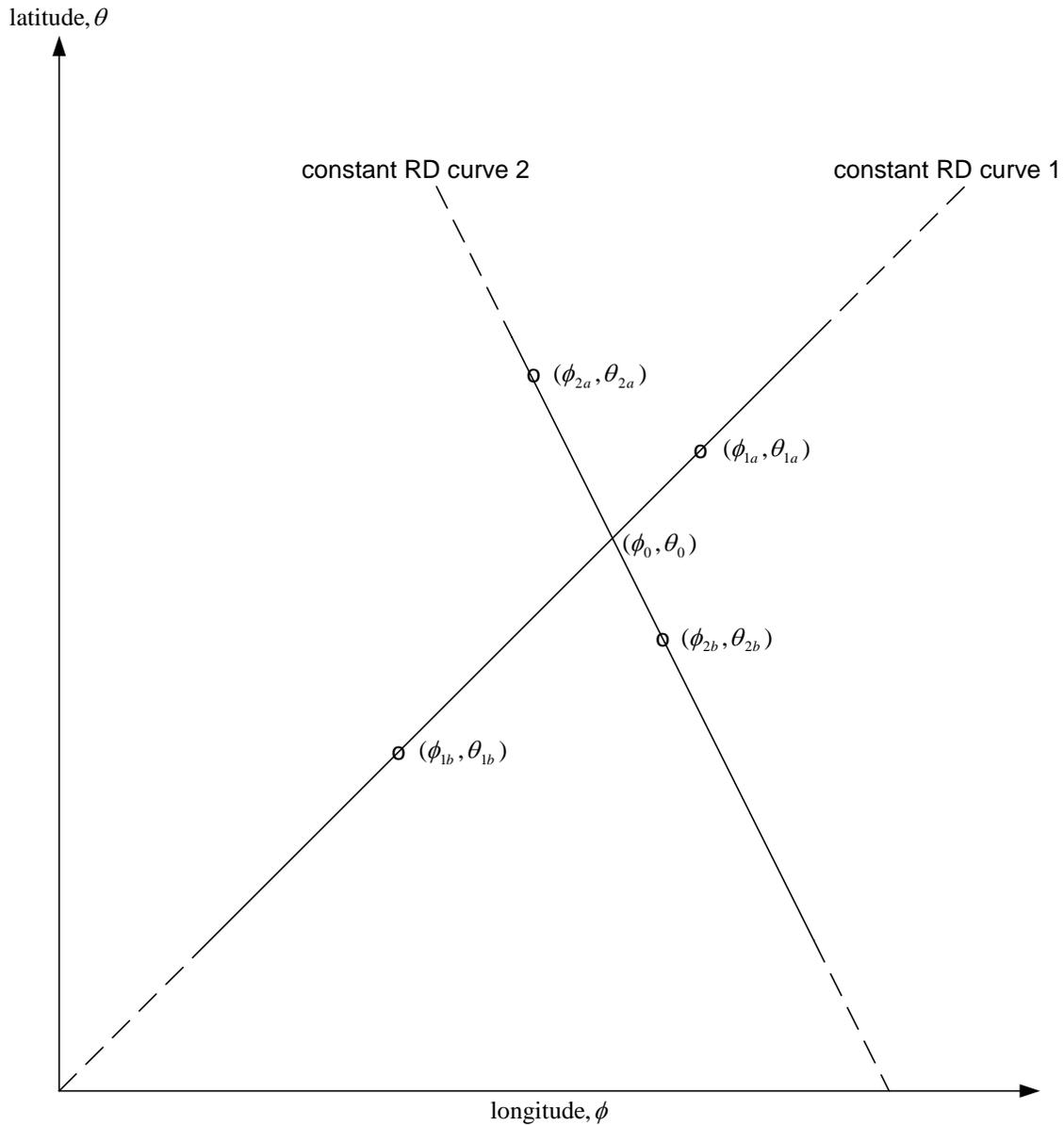
Figure 7: Two constant range-difference curves in the neighbourhood of their intersection point, showing the longitude and latitude of the points just before and just after intersection for each of the two curves.
