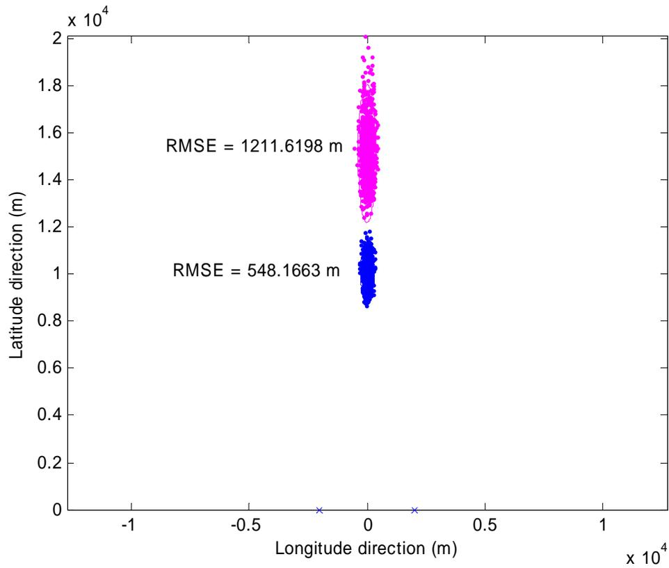
Figure 8: Comparison of location estimates for two emitter positions along the perpendicular bisector of the line joining two receiver pairs. The “x” plot symbols mark the two receiver pairs separated by 4 km. The blue dots and ellipse show the 1000 estimates and the 95% concentration ellipse for an emitter at 10 km from the midpoint of the line joining the two receiver pairs. The corresponding estimates for an emitter at 15 km are shown in magenta.
