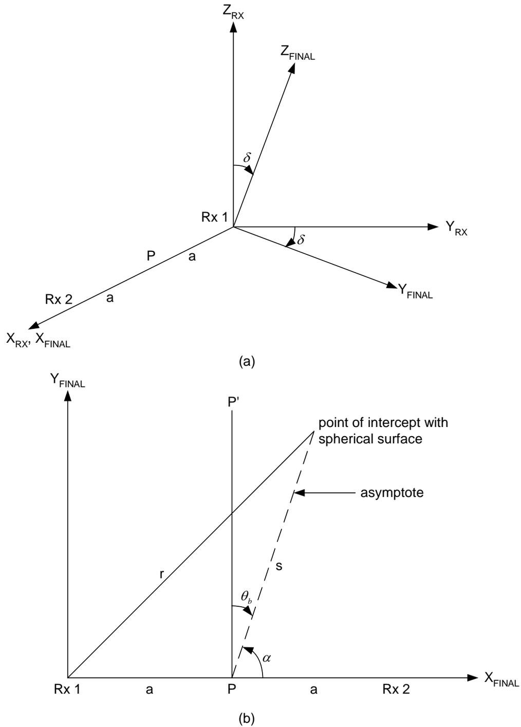
Figure 2: (a) Relation between RX and FINAL coordinate systems; (b) xy-plane of FINAL coordinate system.
