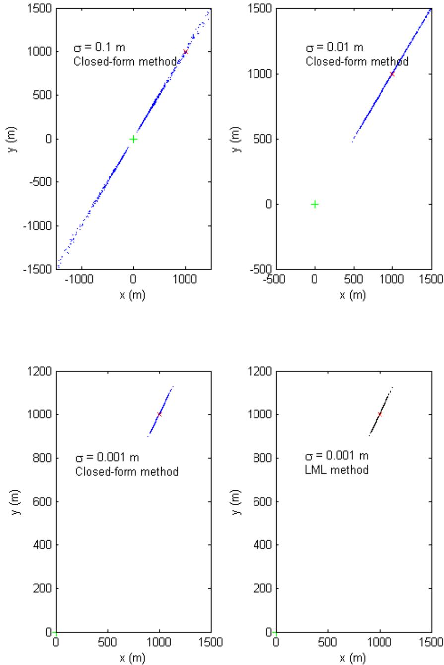
Figure 14: Emitter position estimates on the  $xy$ -plane for the five-receiver array of Figure 11(a), with adjacent-receiver spacing of 10 m, and with emitter at  $(1000, 1000, 0)^T$  m. The top left, top right and bottom left panels show estimates from the closed-form method for  $\sigma = 0.1$  m,  $\sigma = 0.01$  m and  $\sigma = 0.001$  m, respectively. The bottom right panel shows the estimates from the LML method for  $\sigma = 0.001$  m.
