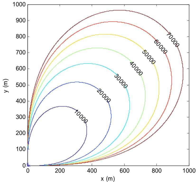
Figure 15: Contours of constant ratio of RMS error to range measurement error standard deviation for two-dimensional emitter geolocation by the LML method. The three receivers are marked by the “x” plot symbols at the origin. The spacing between adjacent receivers is 10 m.
