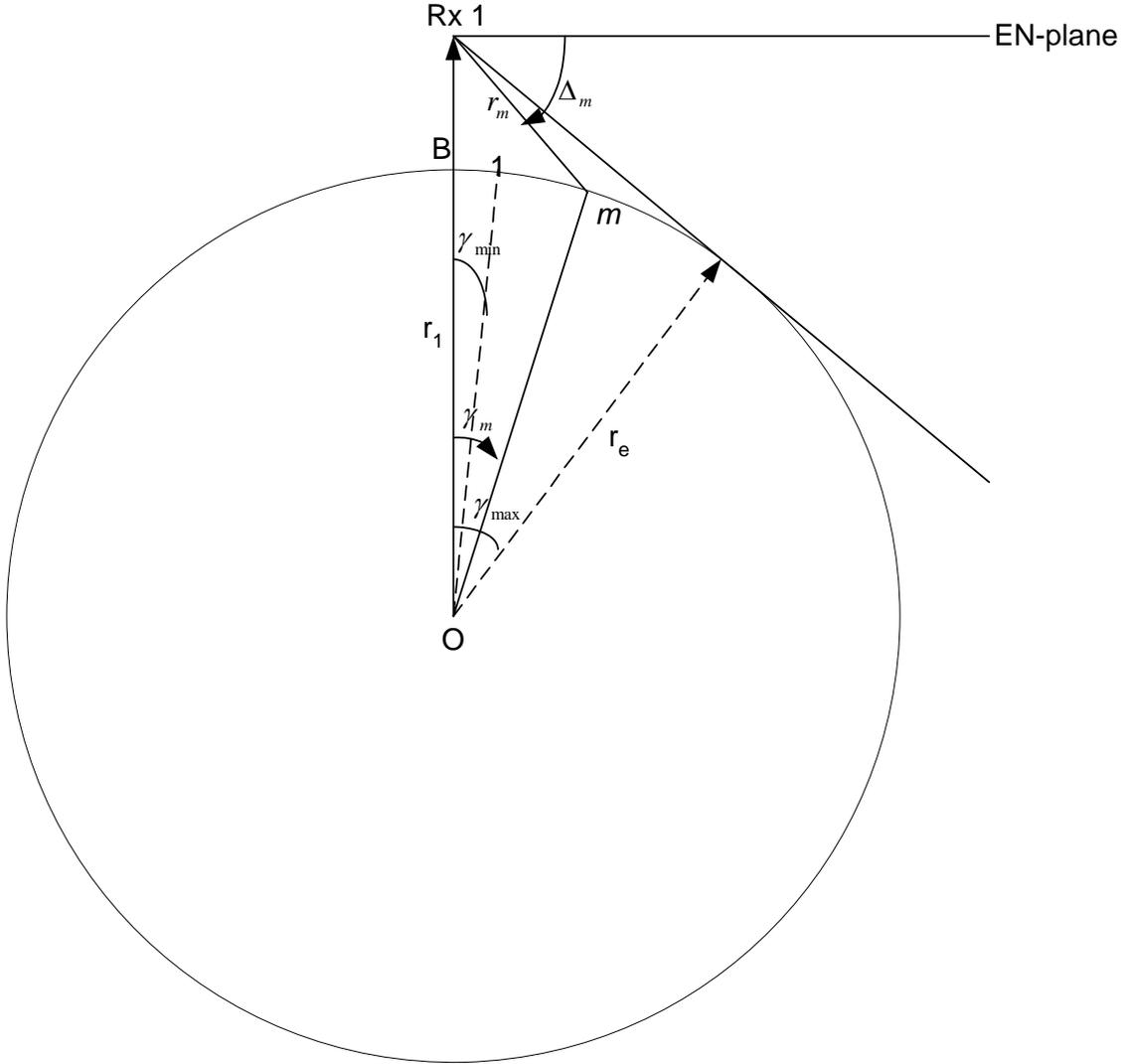
Figure 5:  $M$  equally-spaced points on a circumference passing through receiver 1, showing the angle subtended by the  $m$ th point,  $\gamma_m$ , and the associated slant range  $r_m$  and depression angle  $\Delta_m$ .
