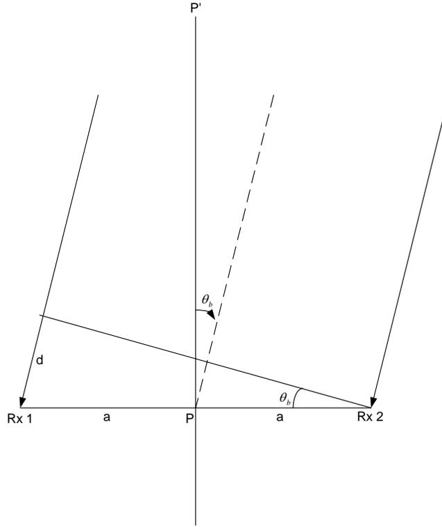
Figure 4: The lines joining two receivers to a distant emitter, showing the relation between the range difference,  $d$ , and the bearing,  $\theta_b$ .
