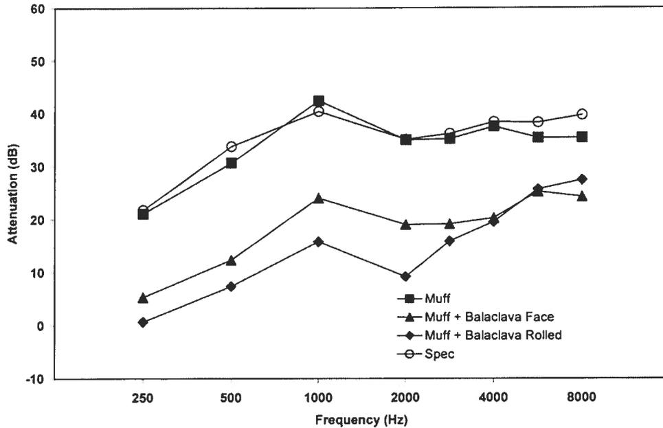
Fig. 3. Effects of the three protector conditions on sound attenuation. Spec, manufacturer's specifications.
