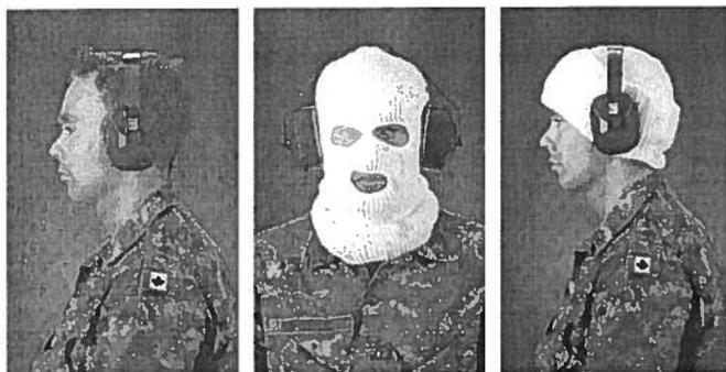
Fig. 1. E-A-R 3000 earmuffs worn alone (left) or with a balaclava full face (center) or rolled (right).
