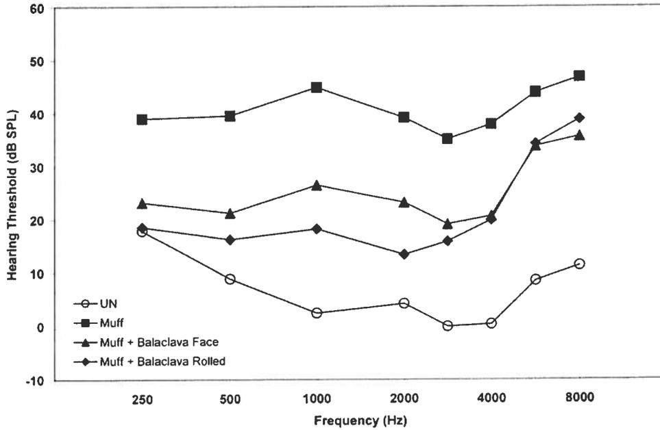
Fig. 2. Effects of the four ear conditions on hearing thresholds. UN, unoccluded.
