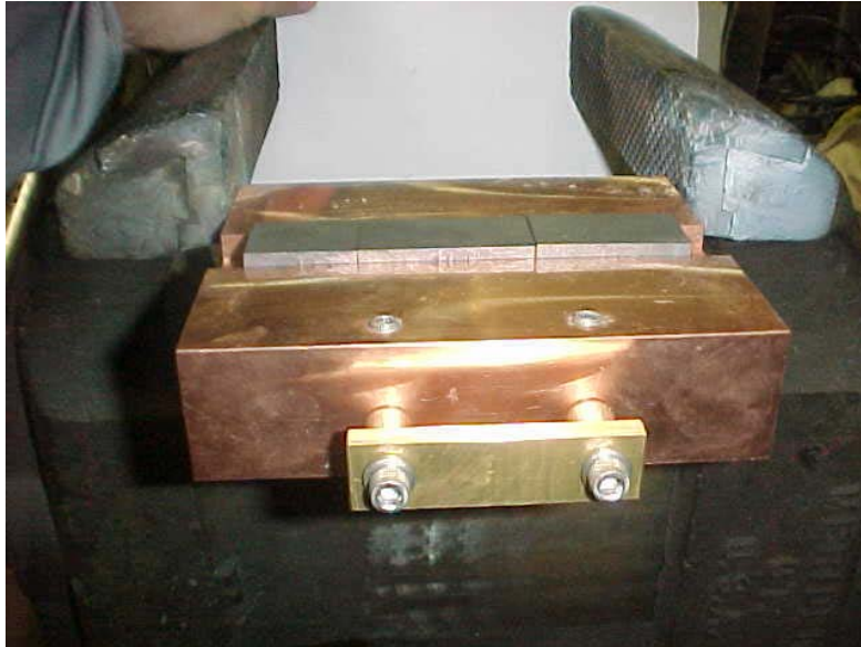
Figure 1. Clamping fixture used to hold weld test assemblies
