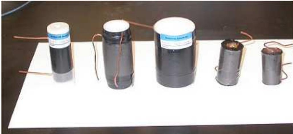
**Figure 7.** Rolled dielectric actuators fabricated from silicone and polyurethane dielectric layers.
