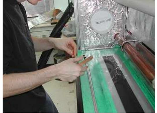
**Figure 5.** Apparatus for fabrication of rolled dielectric actuators.
