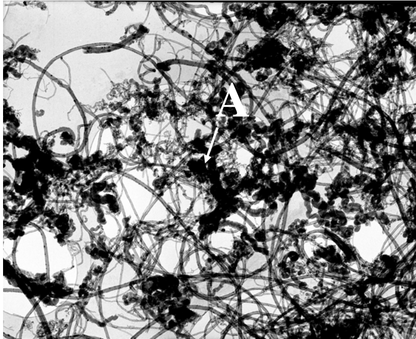
Figure 1. TEM Image of As-Received MWNT
