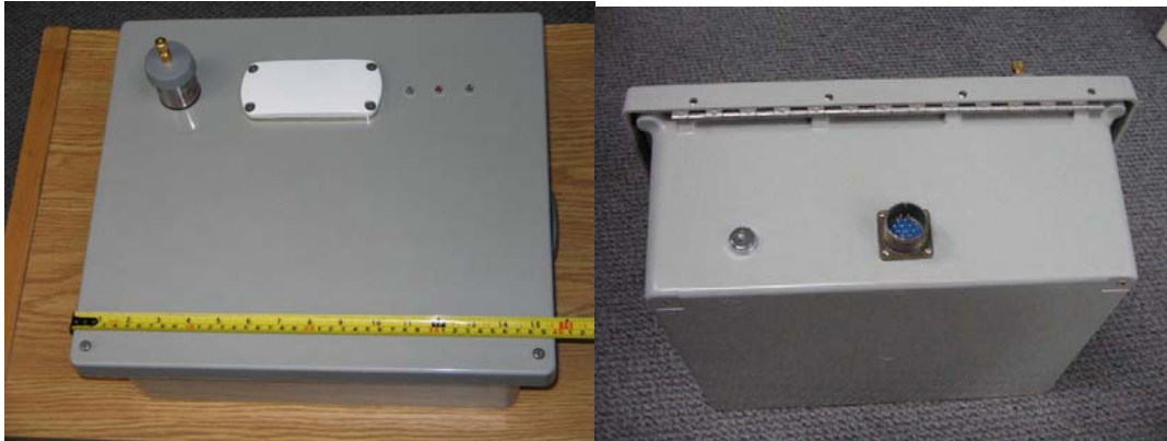
Figure 6. Top (a) and side (b) views of an AVMS remote station. The top view shows the VHF antenna mount and the white, combined Iridium/GPS antenna, while the side view shows the key driven power switch and the connector for the electrical power. This connector also functions as an Ethernet or serial port. A cable integrating these three functions would be supplied with the unit.
