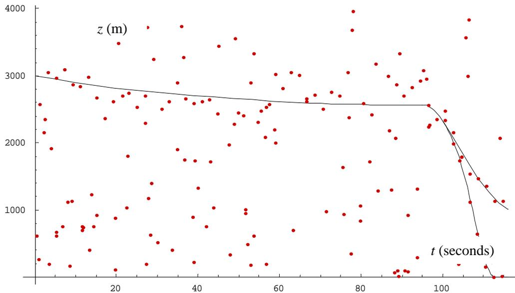
**Figure 5.** Ground truth and radar contacts in Scenario Four – altitude ( $z$ ) versus time ( $t$ )
