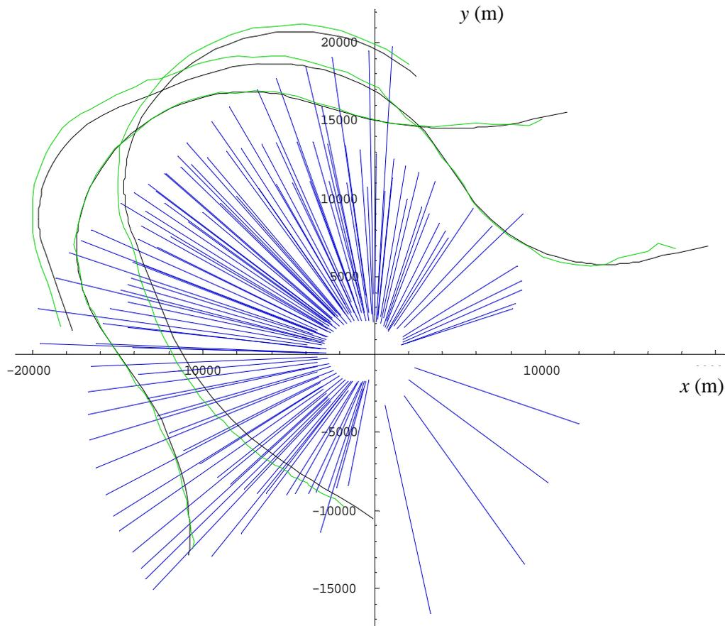
**Figure 12.** Ground truth, radar tracks, and IRST contacts in Scenario Nine – 2D positions
