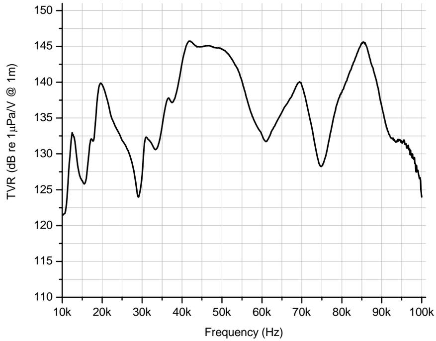
Figure 2 HF MMPP endfire transmitting voltage response.
