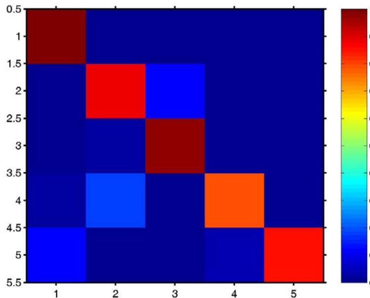
*Figure 17 Confusion Matrix resulting from the nearest neighbour classification of the 5 echo classes: (1) fibreglass plate background (2) basic “mine” (3) basic “mine” with thin aluminum disc (4) basic “mine” with thin aluminum disc and sphere on top and (5) basic “mine” with thin and thick aluminum discs on top.*
