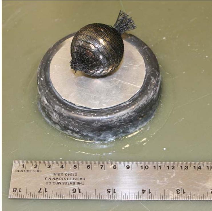
Figure 11 40 mm tungsten carbide sphere atop “mine” and thin aluminum plate.
