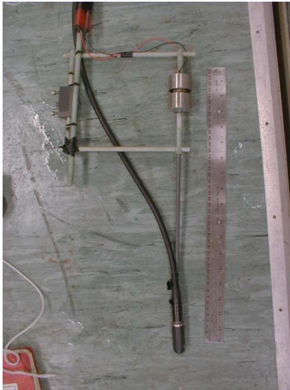
Figure 3 Detail of HF MMPP and hydrophone jig.
