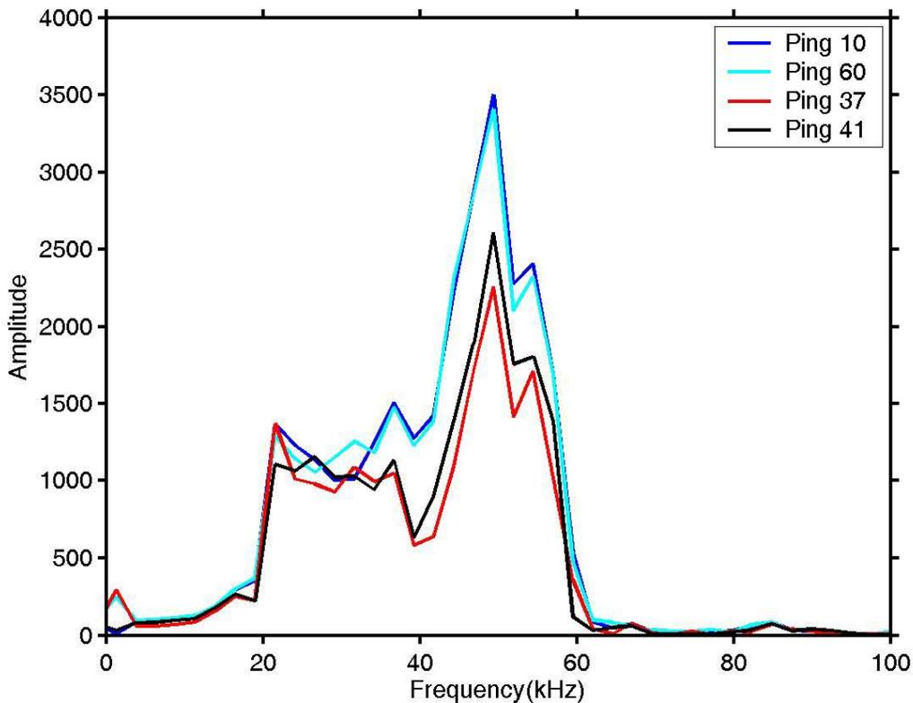
Figure 7 Representative spectra of pings over the fibreglass (blue, cyan) and pings over the “mine” region (red, black).
