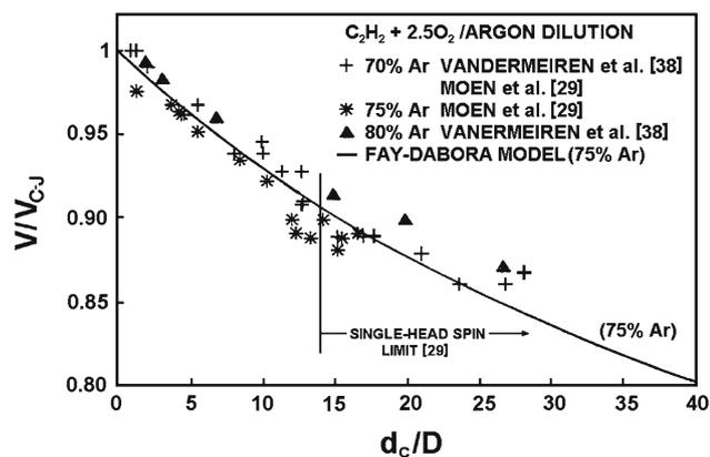
**Fig. 14** Measured detonation velocity,  $V/V_{C-J}$ , versus mixture sensitivity,  $d_c/D$ , in single smooth-walled tubes and channels for stoichiometric acetylene–oxygen mixtures highly diluted with argon [19]; reproduced with permission of the American Institute of Astronautics and Aeronautics
