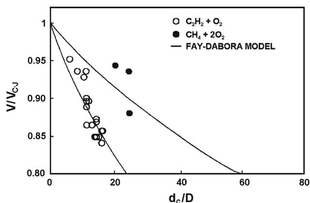
**Fig. 15** Measured detonation velocity,  $V/V_{C-J}$ , versus mixture sensitivity,  $d_c/D$ , in smooth-walled glass tube bundles for equimolar acetylene–oxygen and stoichiometric methane–oxygen [19]; reproduced with permission of the American Institute of Astronautics and Aeronautics
