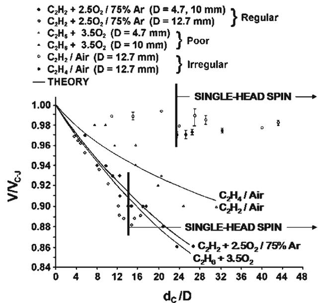
Fig. 13 Detonation velocity,  $V/V_{C-J}$ , versus mixture sensitivity,  $d_c/D$ , for mixtures having different levels of cellular regularity as reported by Moen et al. [29]. The solid curves are calculations based on the Fay-Dabora model [6, 13]; reproduced with permission of DRDC Suffield
