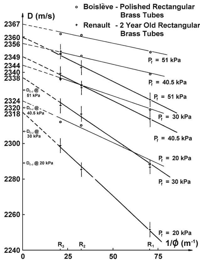
**Fig. 2** Detonation velocity versus  $\phi^{-1}$  for polished and rough brass tubes of rectangular cross section for stoichiometric  $C_3H_8-O_2$  mixtures at 292 K [34]. The arrows along the vertical axis indicate the theoretical detonation velocity for each initial pressure; courtesy of G. Renault
