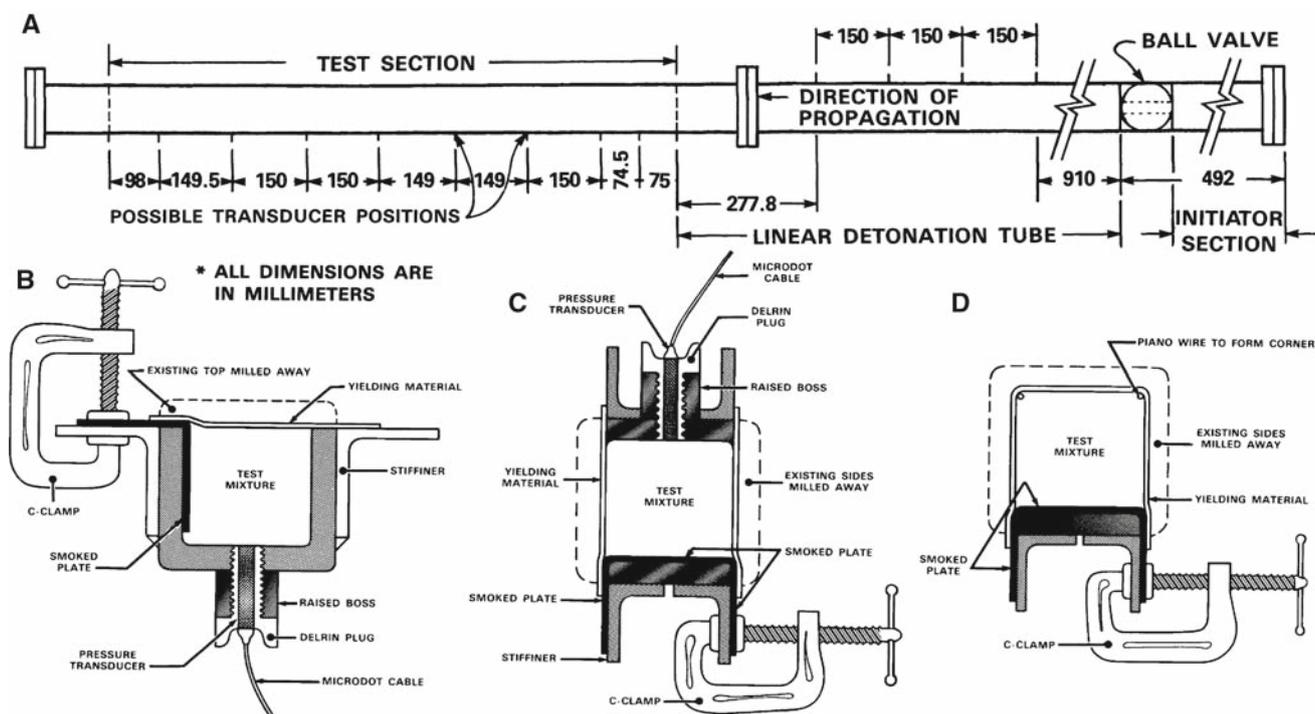
**Fig. 9** Apparatus used to investigate critical conditions and velocity deficits resulting from yielding confinement. A schematic diagram of the detonation tube is shown at the *top*. Test sections with one, two, and three yielding walls are shown from *left* to *right*, respectively
