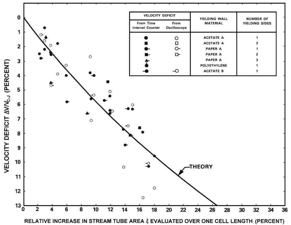
**Fig. 12** Measured velocity deficits,  $\Delta V/V_{C-J}$ , as a function of the calculated stream tube area increase,  $\xi$ , evaluated over one cell length,  $L_c$ , based on the data for rigid tubes from Manson's students, and the data of others researchers [31,32]
