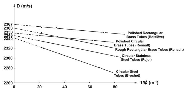
**Fig. 4** A compilation of detonation velocity results for tubes of rectangular and circular cross section having various surface finishes. The mixtures were  $C_3H_8-O_2$  at 292 K and 51 kPa [34]; courtesy of G. Renault
