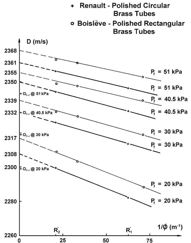
**Fig. 3** Detonation velocity versus  $\phi^{-1}$  for polished brass tubes of circular and rectangular cross section for stoichiometric  $C_2H_4-O_2$  mixtures at 292 K [34]. The arrows along the vertical axis indicate the theoretical detonation velocity for each initial pressure; courtesy of G. Renault
