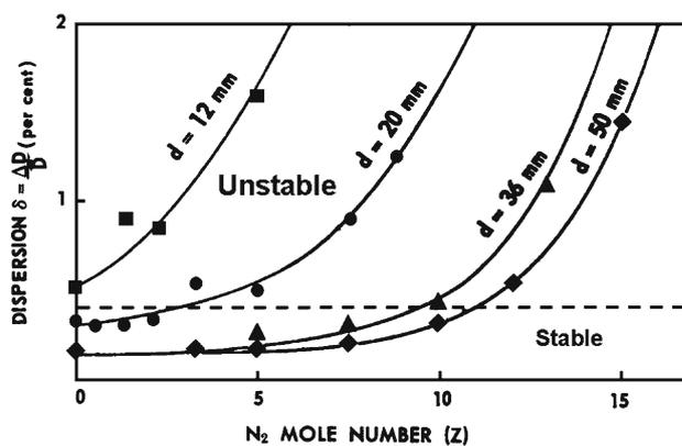
**Fig. 5** Relative dispersion,  $\delta$ , versus nitrogen mole number,  $Z$ , for  $C_3H_8 + 5O_2 + ZN_2$ ,  $P_o = 101.3$  kPa and  $T_o = 298$  K [24]; reproduced with permission of the Combustion Institute
