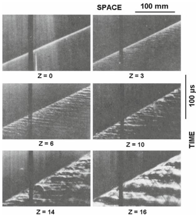
**Fig. 6** Streak schlieren photographs of detonations showing instability evolution in  $\text{C}_3\text{H}_8 + 5\text{O}_2 + \text{ZN}_2$  mixtures as  $Z$  increases;  $d = 20$  mm,  $P_o = 101.3$  kPa,  $T_o = 298$  K [24]; reproduced with permission of the Combustion Institute
