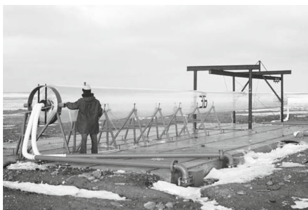
Fig. 7 Apparatus used for the study of critical conditions, velocity deficits, and detonation stability [31,32]
