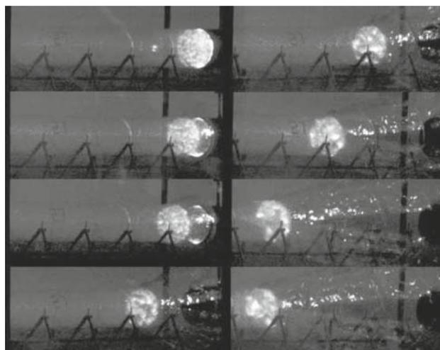
**Fig. 8** Cine frames showing propagation of detonation in a 10-mil plastic tube for 3.90% ethylene–air;  $D/\lambda \cong 4.1$  [31,32]
