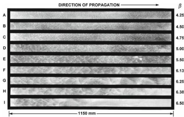
**Fig. 10** Series of smoke records from a square channel having three rigid walls and one yielding acetate wall. The records appear in order of decreasing mixture sensitivity with marginal conditions apparent for  $\beta = 6.25$
