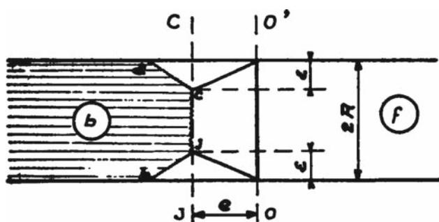
**Fig. 1** Model of the detonation wave with wall effects proposed by Manson and Guénoche [25]; reproduced with permission of the Combustion Institute
