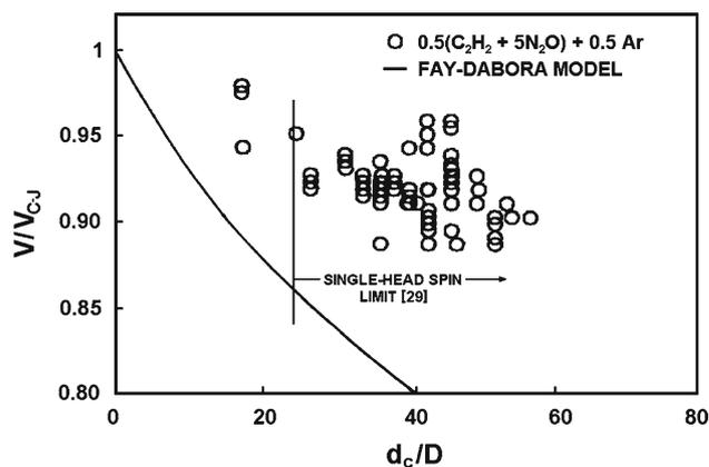
**Fig. 16** Measured detonation velocity,  $V/V_{C-J}$ , versus mixture sensitivity,  $d_c/D$ , in smooth-walled glass tubes for a detonable mixture characterized by a highly irregular cellular structure [19]; reproduced with permission of the American Institute of Astronautics and Aeronautics
