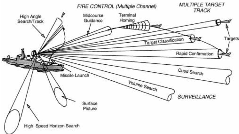
Figure 1: Multiple tasks of typical ship-borne radar systems [7].
